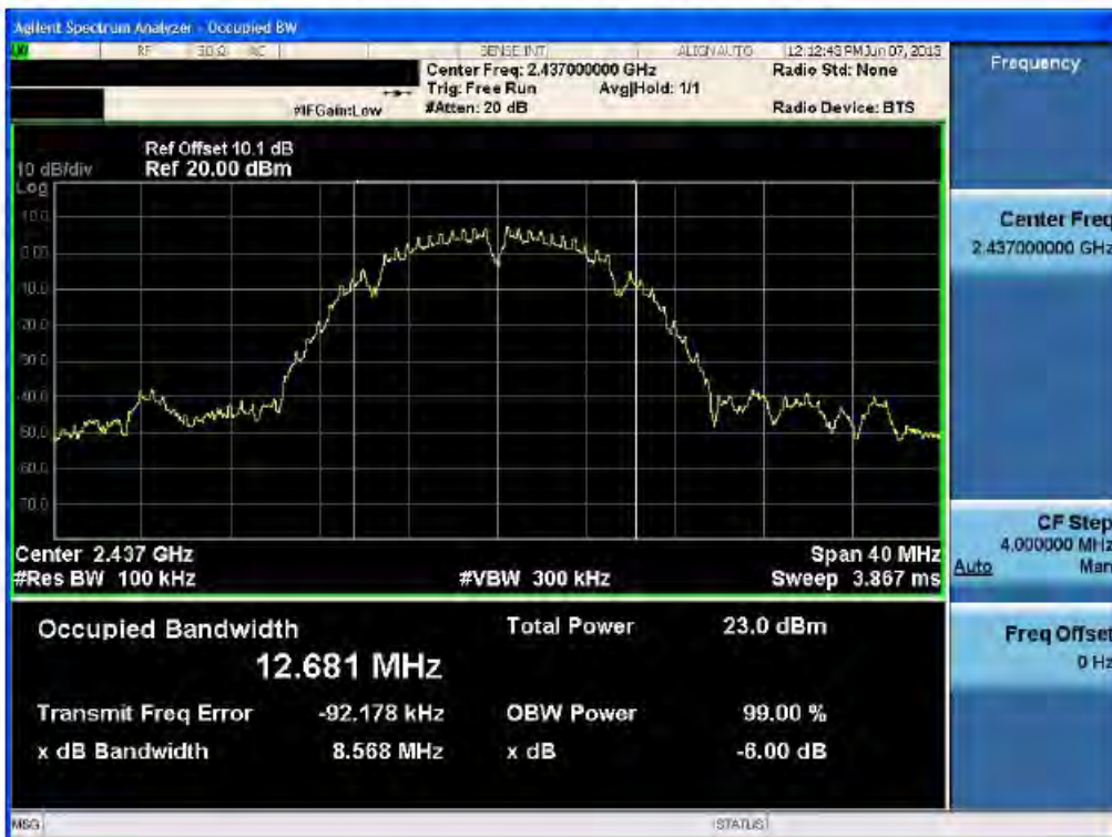
6dB Bandwidth plot (802.11b-CH 6)
