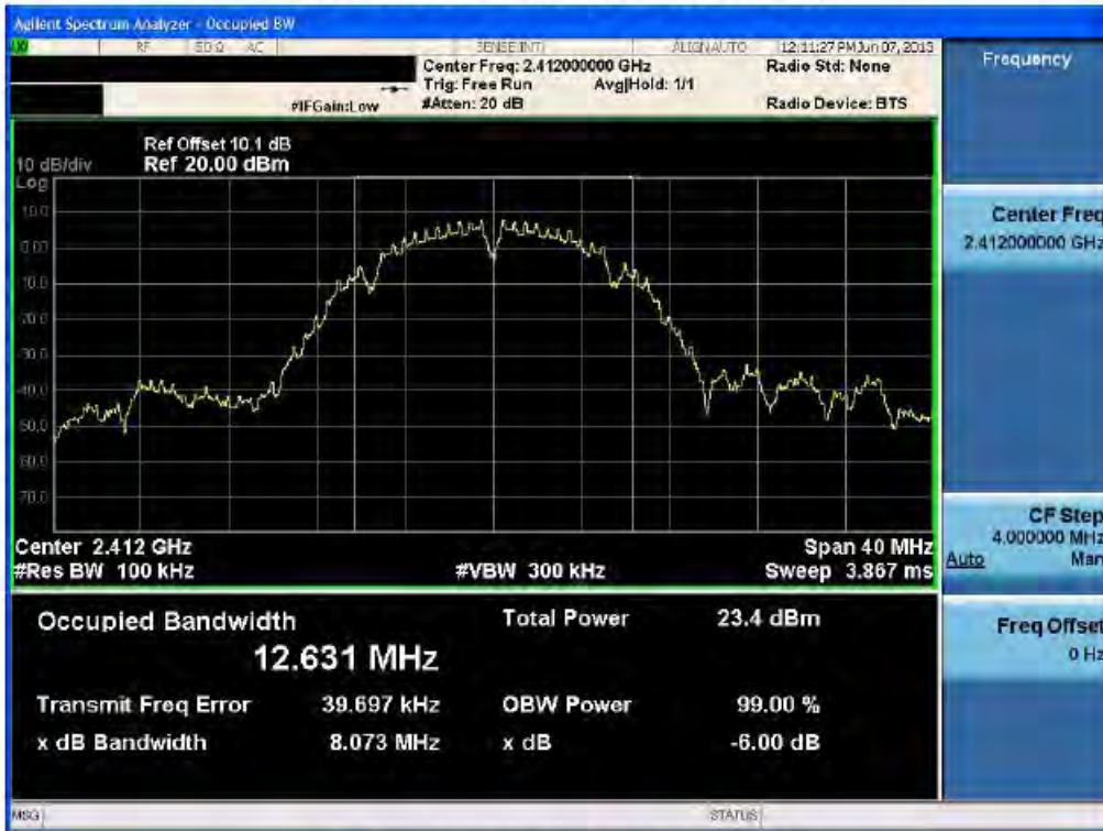
6dB Bandwidth plot (802.11b-CH 6)
