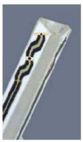
Figure 3.3 Probe Thick-Film Technique
