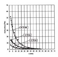
Figure 3.5 E-Field and Temperature Measurements at 1800MHz
