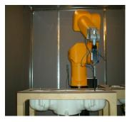
Figure 4.1 DASY4 Test System
