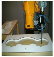
(HEC) gelling agent and saline solution (see Table 3.1). Preservation with a bactericide is added and visual inspection is made to make sure air bubbles are not trapped during the mixing process. The mixture is calibrated to obtain proper dielectric constant (permittivity) and conductivity of the desired tissue. The mixture characterizations used for the brain and muscle tissue simulating liquids are according to the data by C. Gabriel and G. Harts grove.
