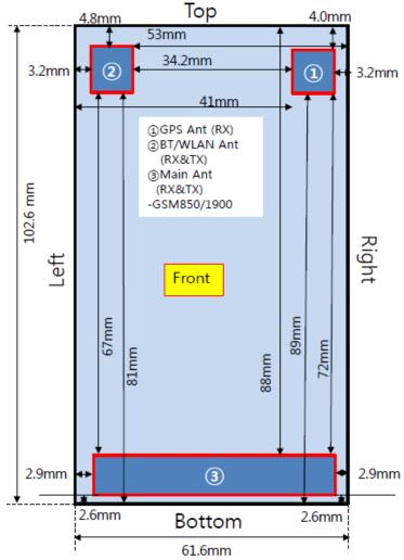
Figure 13.1 Identification of Sides for SAR Testing
