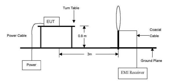
The diagram below shows the test setup that is utilized to make the measurements for emission .The spurious emissions were investigated form 30 MHz to 1 GHz.
