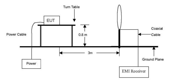
The diagram below shows the test setup that is utilized to make the measurements for emission from 30  $\,\text{Mb}$  to 1  $\,\text{GHz}$  Emissions.
