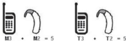
In the above example, if a hearing aid meets the M2 level rating and the wireless phone meets the M3 level rating, the sum of the two values equal M5. This should provide the hearing aid user with "normal usage" while using their hearing aid with the particular wireless phone. "Normal usage" in this context is defined as a signal quality that's acceptable for normal operation.
