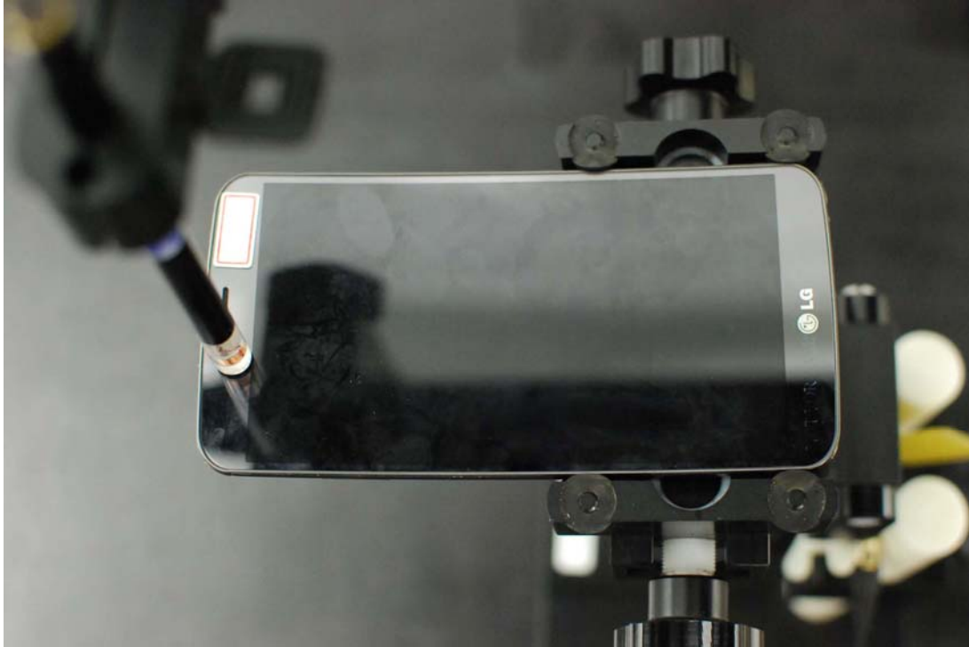
Figure 13-1 Test Setup for Wireless Device
