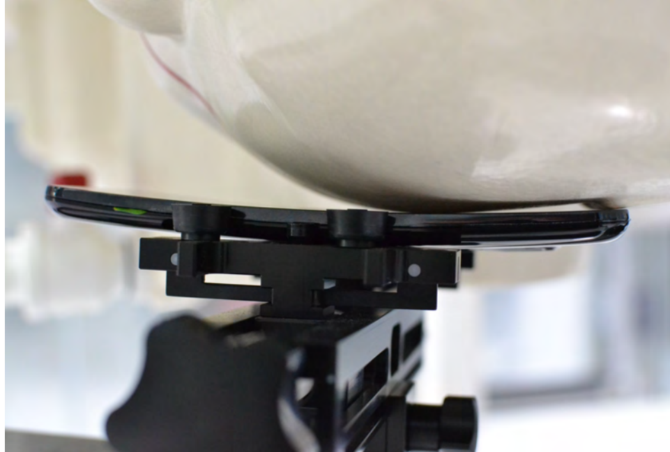
SAR Test Setup Photo 3 - Left Cheek
