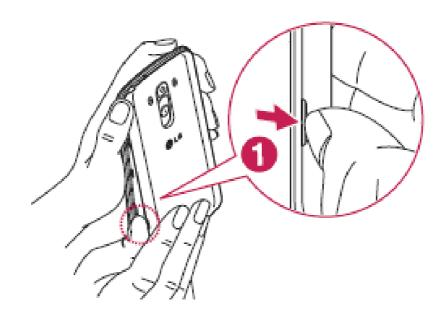
2 Slide the SIM card into the lower slot for the SIM card as shown in the fi gure. Make sure the gold contact area on the card is facing downwards.
