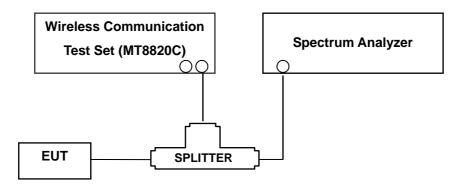
(Configuration of conducted Emission measurement)
