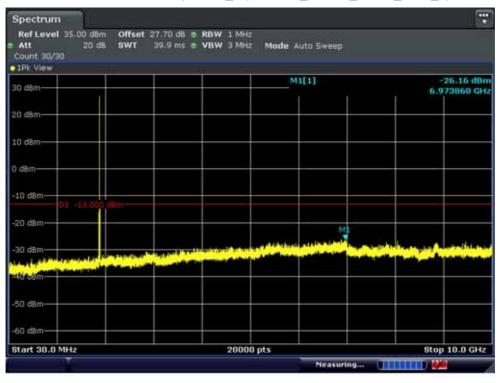
BAND 2. Conducted Spurious\_1 (19125ch\_15MHz\_QPSK\_RB 1\_0)
