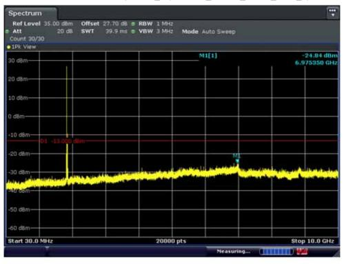
BAND 2. Conducted Spurious\_1 (18700ch\_20MHz\_QPSK\_RB 1\_0)
