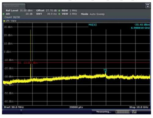
BAND 2. Conducted Spurious\_1 (19150ch\_10MHz\_QPSK\_RB 1\_0)
