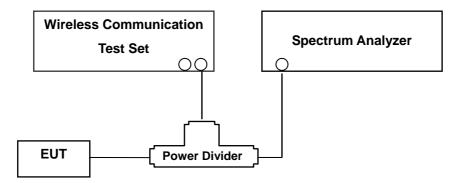
(Configuration of conducted Emission measurement)
