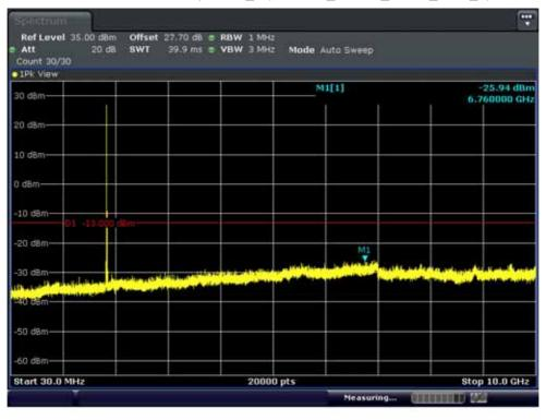
BAND 2. Conducted Spurious\_1 (18650ch\_10MHz\_QPSK\_RB 1\_0)
