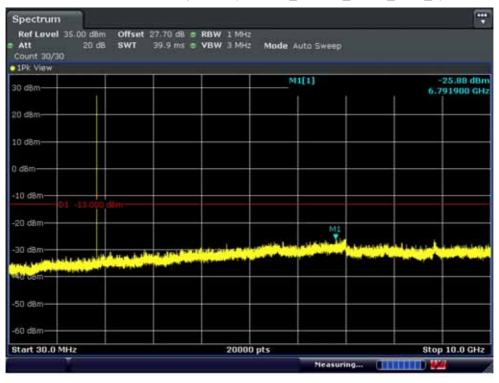
BAND 2. Conducted Spurious (18607ch\_1.4MHz\_QPSK\_RB 1\_0)
