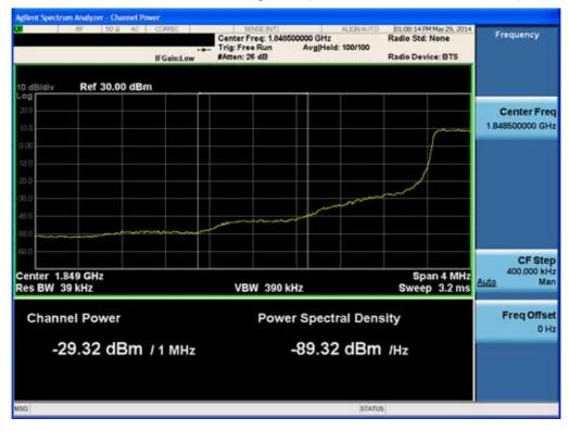
BAND 2. Lower Extended Band Edge Plot (1.4M BW Ch.18607 QPSK RB 6) -3
