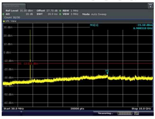
BAND 2. Conducted Spurious (18625ch\_5MHz\_QPSK\_RB 1\_0)
