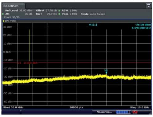
BAND 2. Conducted Spurious (18615ch\_3MHz\_QPSK\_RB 1\_0)
