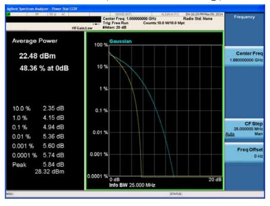
BAND 2. PAR Plot (20M BW Ch.18900 QPSK RB 100\_0)
