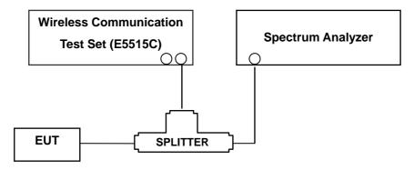
(Configuration of conducted Emission measurement)
