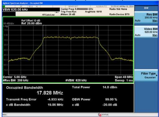
20 dB Bandwidth plot (802.11n\_40 MHz BW-CH 134)
