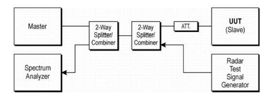
Figure 3-1. Conducted Test Setup for DFS
