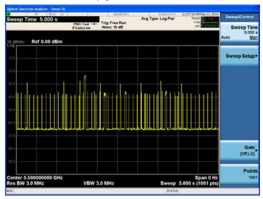
Time Display, WLAN Channel Traffic (Streaming Video)
