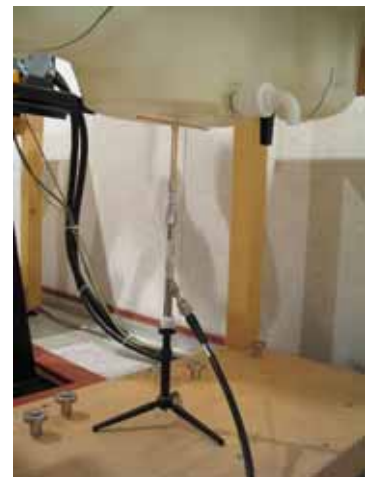
Photo of the dipole Antenna
