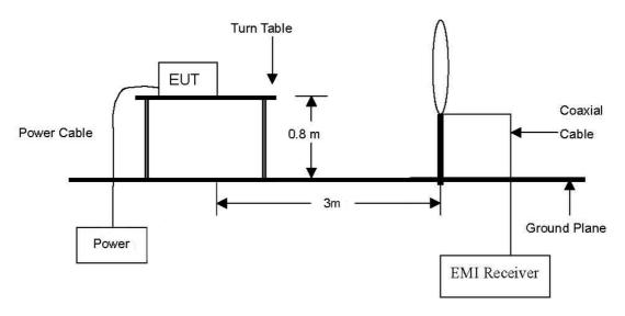
The diagram below shows the test setup that is utilized to make the measurements for emission . The spurious emissions were investigated form 1  $\times$  to the 10th harmonic of the highest fundamental frequency or 40  $\times$ , whichever is lower.
