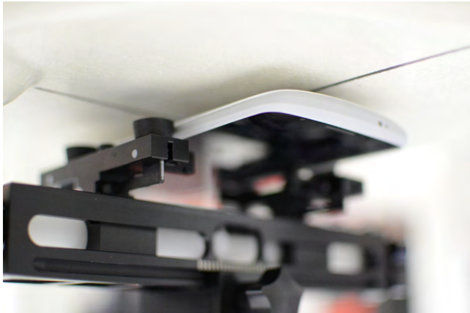
SAR Test Setup Photo 16: Back Side with Wireless Charging Back Cover at 1.0 cm
