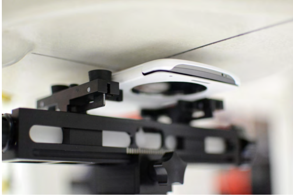
SAR Test Setup Photo 15: Back Side with Folio Accessory, Closed at 1.0 cm
