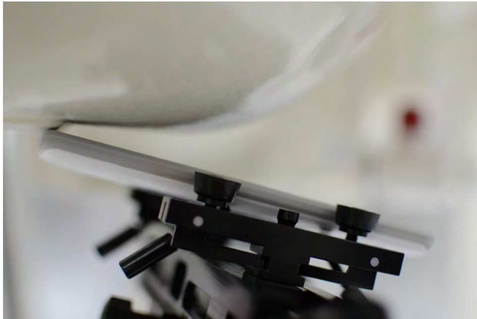
SAR Test Setup Photo 8: Right Tilt with Wireless Charging Back Cover
