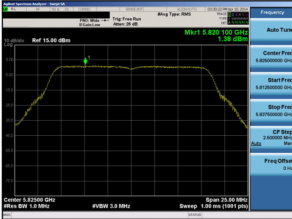
Plot 6-74. Peak Power Spectral Density Plot (802.11a (UNII Band 3) – Ch. 165)
