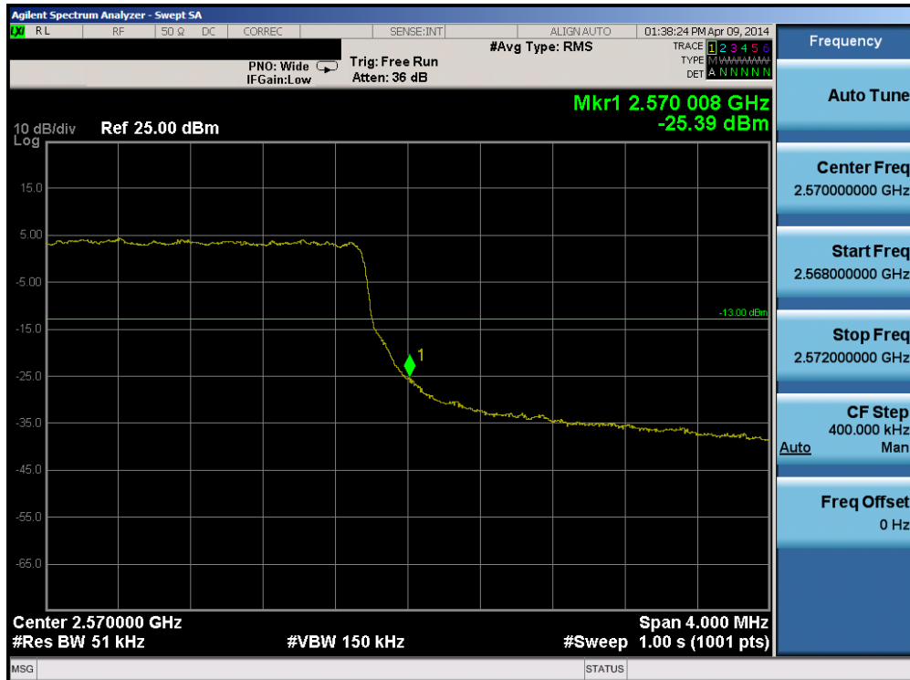
Plot 6-136. Upper Band Edge Plot (Band 7 – 5.0MHz QPSK – RB Size 25)
