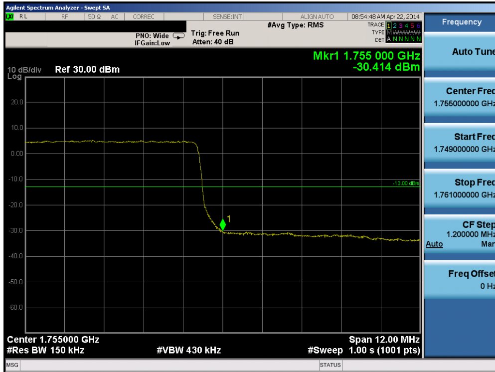
Plot 6-113. Upper Band Edge Plot (Band 4 – 15.0MHz QPSK – RB Size 75)
