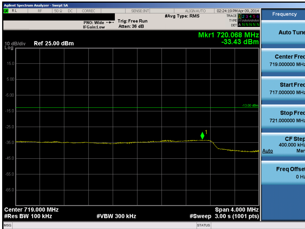
Plot 6-100. Upper Extended Band Edge Plot (Band 17 – 5.0MHz QPSK – RB Size 25)
