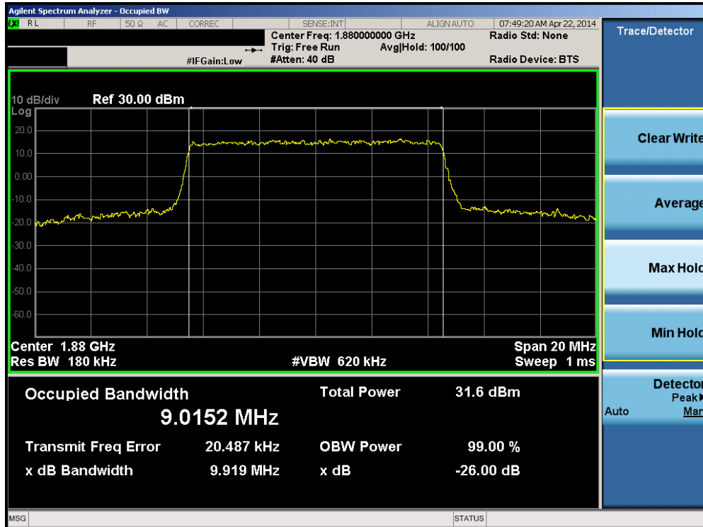
Plot 6-15. Occupied Bandwidth Plot (Band 2 – 10.0MHz QPSK – RB Size 50)
