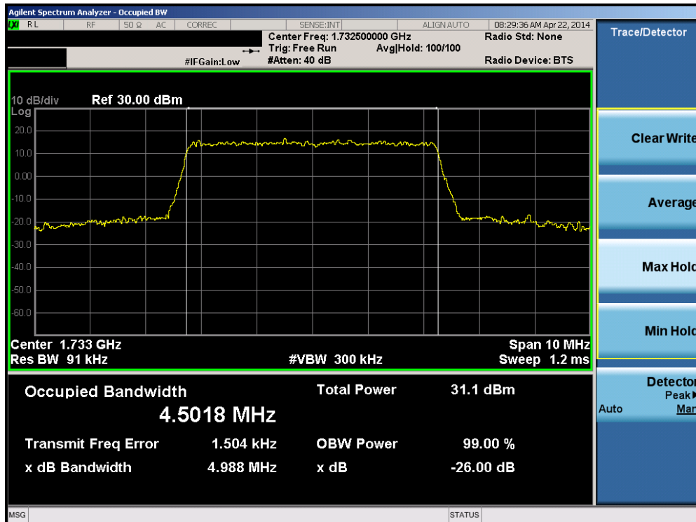
Plot 6-6. Occupied Bandwidth Plot (Band 4 – 5.0MHz 16-QAM – RB Size 25)
