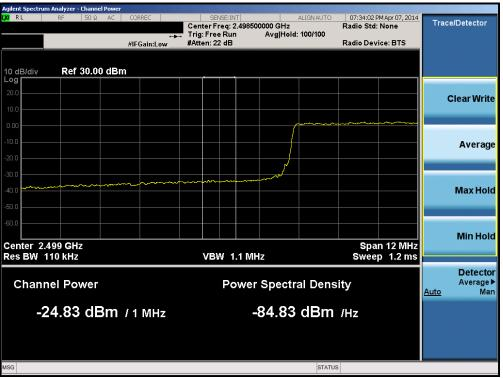
Plot 6-118. Lower Extended Band Edge Plot (Band 7 – 15.0MHz QPSK – RB Size 75)
