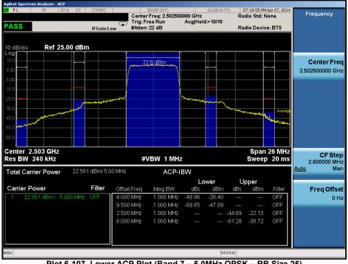
Plot 6-107. Lower ACP Plot (Band 7 – 5.0MHz QPSK – RB Size 25)
