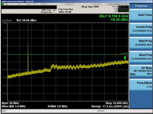
Plot 6-47. Conducted Spurious Plot (Band 4 – 5.0MHz QPSK – RB Size 1, RB Offset 0 – Mid Channel)
