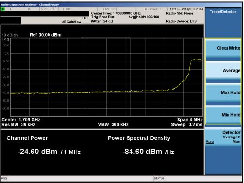
Plot 6-72. Lower Extended Band Edge Plot (Band 4 – 5.0MHz QPSK – RB Size 25)
