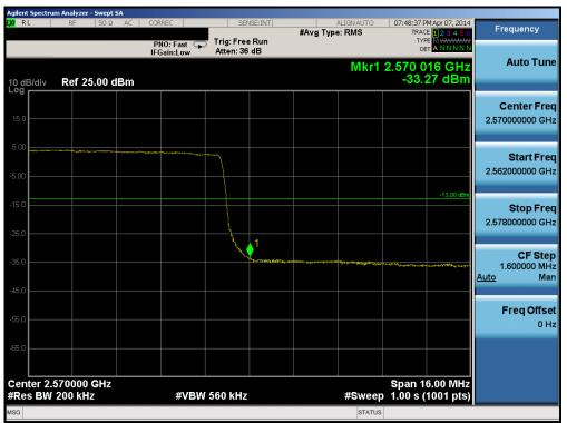
Plot 6-126. Upper Band Edge Plot (Band 7 – 20.0MHz QPSK – RB Size 100)
