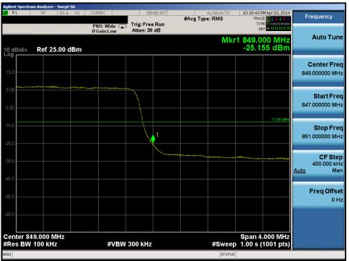
Plot 6-68. Upper Band Edge Plot (Band 5 – 5.0MHz QPSK – RB Size 25)
