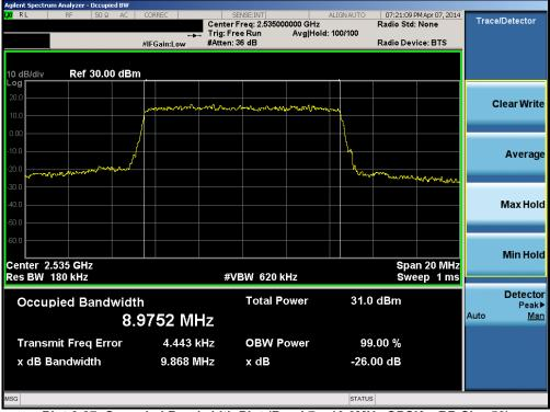
Plot 6-27. Occupied Bandwidth Plot (Band 7 – 10.0MHz QPSK – RB Size 50)
