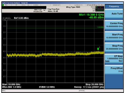
Plot 6-54. Conducted Spurious Plot (Band 2 – 5.0MHz QPSK – RB Size 1, RB Offset 0 – Mid Channel)
