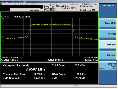
Plot 6-28. Occupied Bandwidth Plot (Band 7 – 10.0MHz 16-QAM – RB Size 50)
