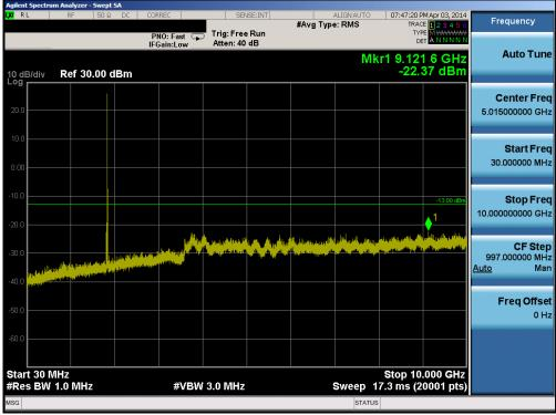
Plot 6-51. Conducted Spurious Plot (Band 2 – 5.0MHz QPSK – RB Size 1, RB Offset 0 – Low Channel)
