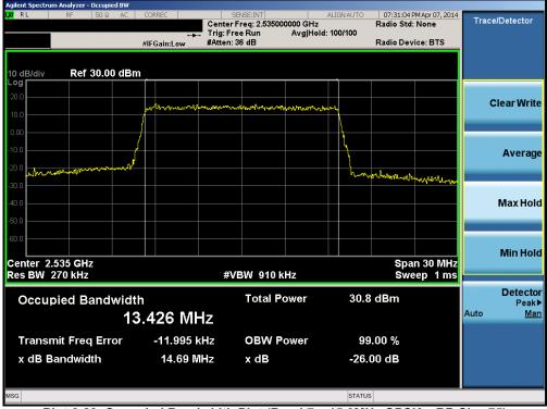
Plot 6-29. Occupied Bandwidth Plot (Band 7 – 15.0MHz QPSK – RB Size 75)
