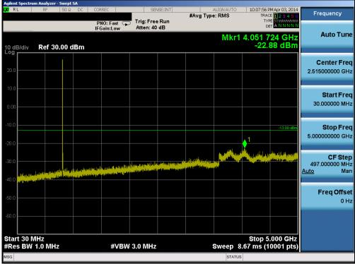
Plot 6-41. Conducted Spurious Plot (Band 5 – 5.0MHz QPSK – RB Size 1, RB Offset 0 – Mid Channel)
