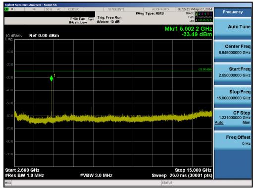
Plot 6-58. Conducted Spurious Plot (Band 7 – 5.0MHz QPSK – RB Size 1, RB Offset 0 – Low Channel)
