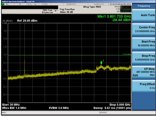
Plot 6-35. Conducted Spurious Plot (Band 17 – 10.0MHz QPSK – RB Size 1, RB Offset 0 – Mid Channel)
