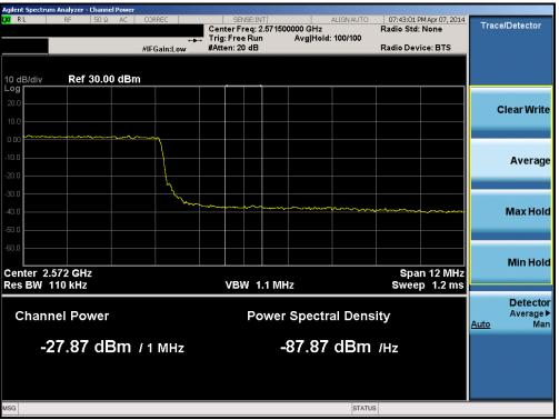
Plot 6-120. Upper Extended Band Edge Plot (Band 7 – 15.0MHz QPSK – RB Size 75)
