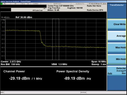
Plot 6-127. Upper Extended Band Edge Plot (Band 7 – 20.0MHz QPSK – RB Size 100)
