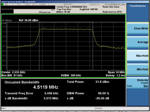
Plot 6-25. Occupied Bandwidth Plot (Band 7 – 5.0MHz QPSK – RB Size 25)
