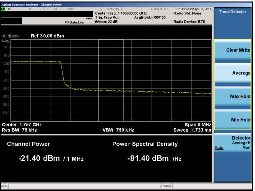
Plot 6-78. Upper Extended Band Edge Plot (Band 4 – 10.0MHz QPSK – RB Size 50)
