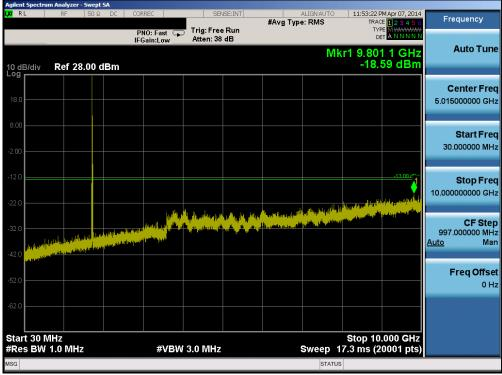
Plot 6-49. Conducted Spurious Plot (Band 4 – 5.0MHz QPSK – RB Size 1, RB Offset 0 – High Channel)
