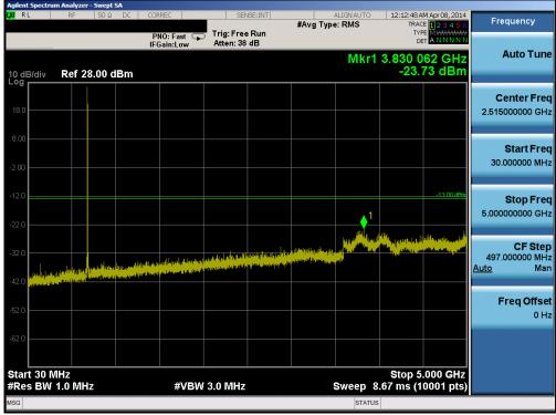
Plot 6-33. Conducted Spurious Plot (Band 17 – 10.0MHz QPSK – RB Size 1, RB Offset 0– Low Channel)
