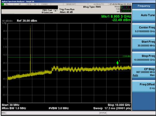
Plot 6-53. Conducted Spurious Plot (Band 2 – 5.0MHz QPSK – RB Size 1, RB Offset 0 – Mid Channel)
