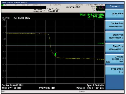
Plot 6-70. Upper Band Edge Plot (Band 5 – 10.0MHz QPSK – RB Size 50)
