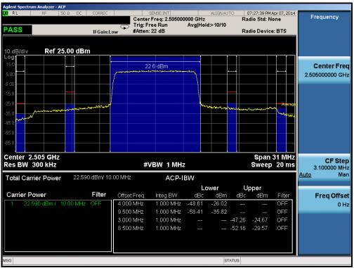
Plot 6-114. Lower ACP Plot (Band 7 – 10.0MHz QPSK – RB Size 50)
