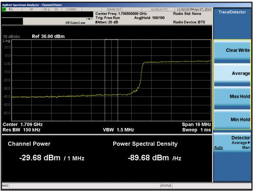
Plot 6-84. Lower Extended Band Edge Plot (Band 4 – 20.0MHz QPSK – RB Size 100)
