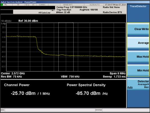
Plot 6-113. Upper Extended Band Edge Plot (Band 7 – 10.0MHz QPSK – RB Size 50)
