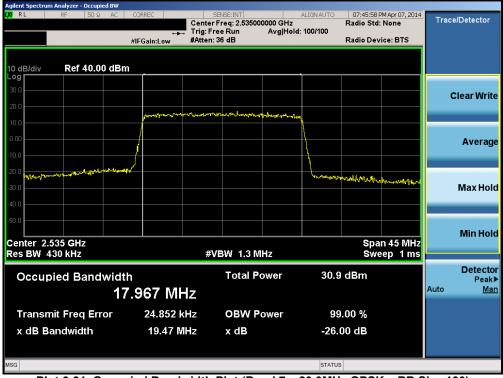
Plot 6-31. Occupied Bandwidth Plot (Band 7 – 20.0MHz QPSK – RB Size 100)
