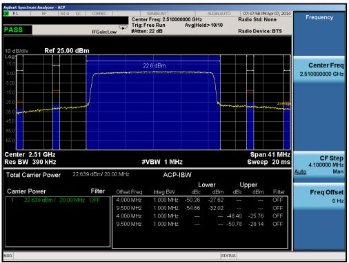
Plot 6-128. Lower ACP Plot (Band 7 - 20.0MHz QPSK - RB Size 100)
