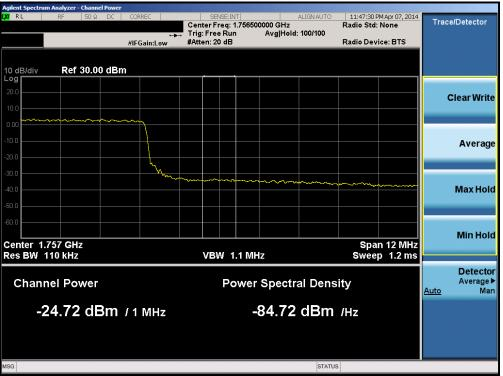
Plot 6-82. Upper Extended Band Edge Plot (Band 4 – 15.0MHz QPSK – RB Size 75)
