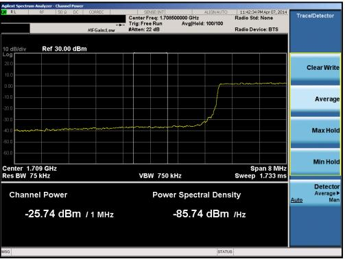
Plot 6-76. Lower Extended Band Edge Plot (Band 4 – 10.0MHz QPSK – RB Size 50)
