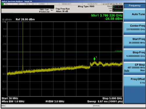
Plot 6-37. Conducted Spurious Plot (Band 17 – 10.0MHz QPSK – RB Size 1, RB Offset 0 – High Channel)
