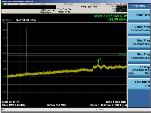
Plot 6-43. Conducted Spurious Plot (Band 5 – 5.0MHz QPSK – RB Size 1, RB Offset 0 – High Channel)
