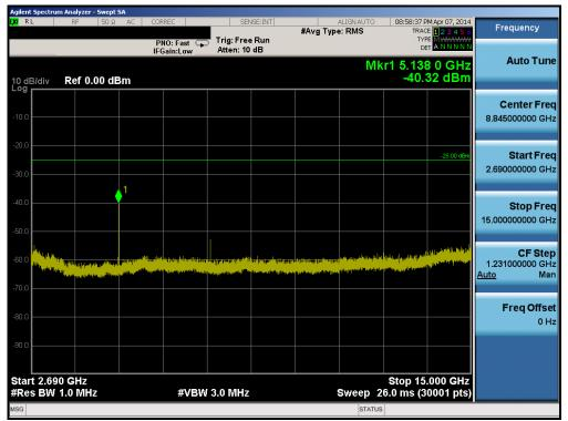
Plot 6-62. Conducted Spurious Plot (Band 7 – 5.0MHz QPSK – RB Size 1, RB Offset 0 – High Channel)
