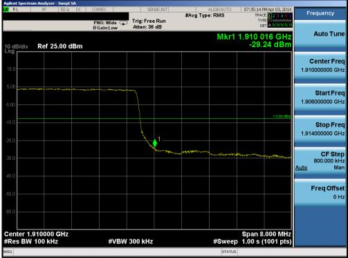
Plot 6-93. Upper Band Edge Plot (Band 2 – 10.0MHz QPSK – RB Size 50)
