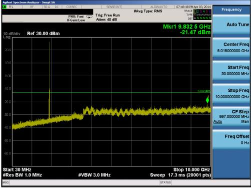
Plot 6-55. Conducted Spurious Plot (Band 2 – 5.0MHz QPSK – RB Size 1, RB Offset 0 – High Channel)
