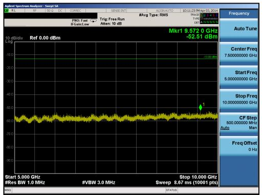
Plot 6-44. Conducted Spurious Plot (Band 5 – 5.0MHz QPSK – RB Size 1, RB Offset 0 – High Channel)
