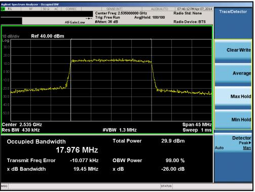
Plot 6-32. Occupied Bandwidth Plot (Band 7 – 20.0MHz 16-QAM – RB Size 100)
