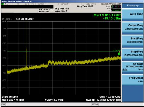
Plot 6-45. Conducted Spurious Plot (Band 4 – 5.0MHz QPSK – RB Size 1, RB Offset 0 – Low Channel)
