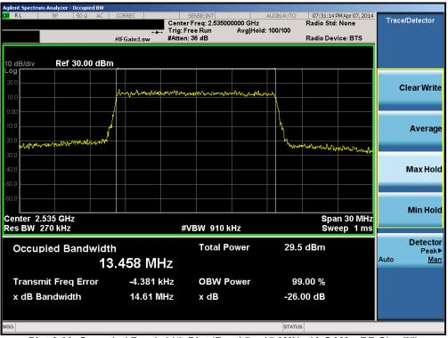
Plot 6-30. Occupied Bandwidth Plot (Band 7 – 15.0MHz 16-QAM – RB Size 75)
