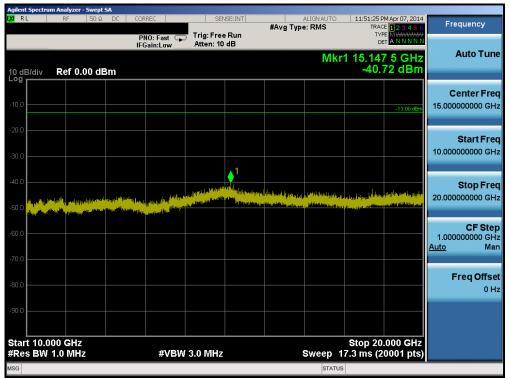
Plot 6-46. Conducted Spurious Plot (Band 4 – 5.0MHz QPSK – RB Size 1, RB Offset 0 – Low Channel)
