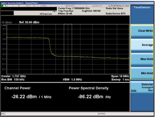
Plot 6-86. Upper Extended Band Edge Plot (Band 4 – 20.0MHz QPSK – RB Size 100)
