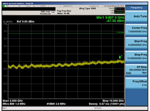
Plot 6-36. Conducted Spurious Plot (Band 17 – 10.0MHz QPSK – RB Size 1, RB Offset 0 – Mid Channel)
