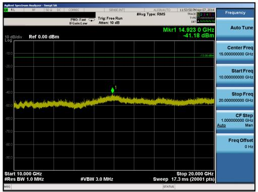
Plot 6-50. Conducted Spurious Plot (Band 4 – 5.0MHz QPSK – RB Size 1, RB Offset 0 – High Channel)
