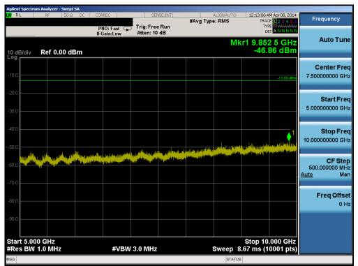
Plot 6-34. Conducted Spurious Plot (Band 17 – 10.0MHz QPSK – RB Size 1, RB Offset 0 – Low Channel)
