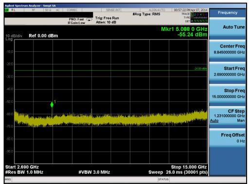
Plot 6-60. Conducted Spurious Plot (Band 7 – 5.0MHz QPSK – RB Size 1, RB Offset 0 – Mid Channel)
