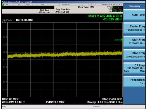
Plot 6-57. Conducted Spurious Plot (Band 7 – 5.0MHz QPSK – RB Size 1, RB Offset 0 – Low Channel)
