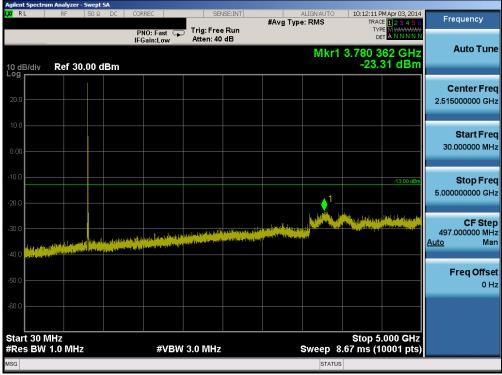
Plot 6-39. Conducted Spurious Plot (Band 5 – 5.0MHz QPSK – RB Size 1, RB Offset 0 – Low Channel)
