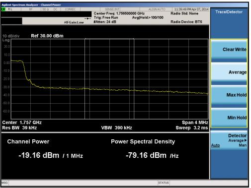
Plot 6-74. Upper Extended Band Edge Plot (Band 4 – 5.0MHz QPSK – RB Size 25)
