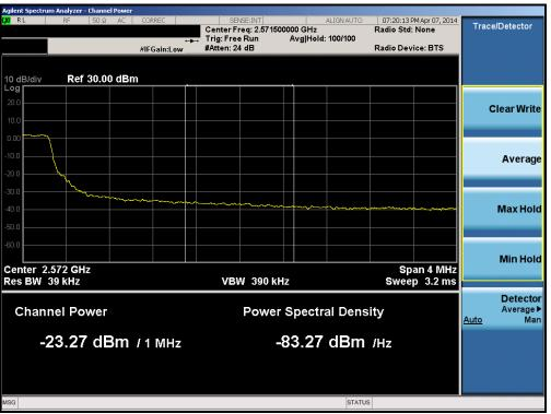
Plot 6-106. Upper Extended Band Edge Plot (Band 7 – 5.0MHz QPSK – RB Size 25)
