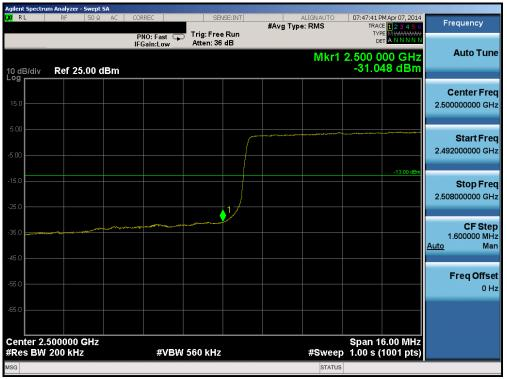
Plot 6-124. Lower Band Edge Plot (Band 7 - 20.0MHz QPSK - RB Size 100)
