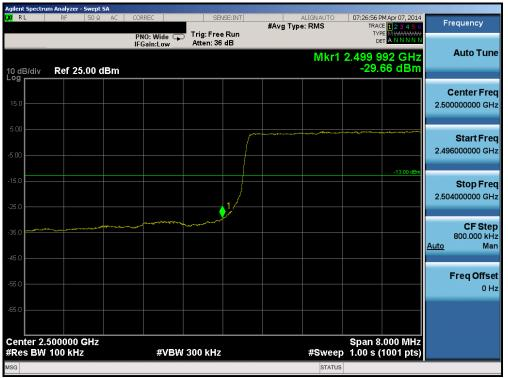
Plot 6-110. Lower Band Edge Plot (Band 7 – 10.0MHz QPSK – RB Size 50)
