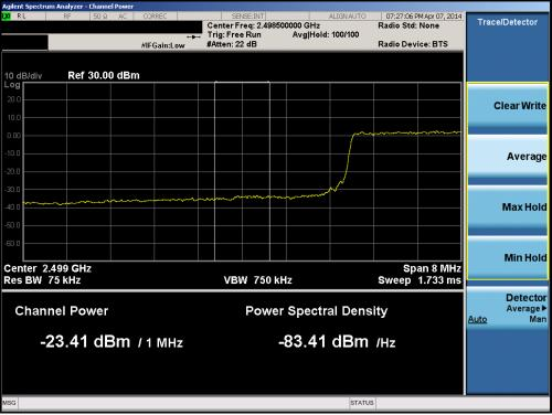
Plot 6-111. Lower Extended Band Edge Plot (Band 7 – 10.0MHz QPSK – RB Size 50)
