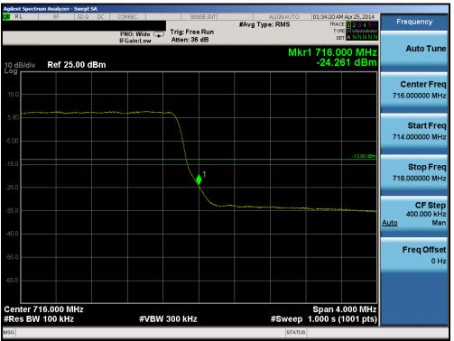
Plot 6-64. Upper Band Edge Plot (Band 17 – 5.0MHz QPSK – RB Size 25)
