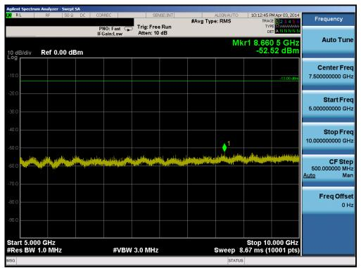
Plot 6-40. Conducted Spurious Plot (Band 5 – 5.0MHz QPSK – RB Size 1, RB Offset 0 – Low Channel)
