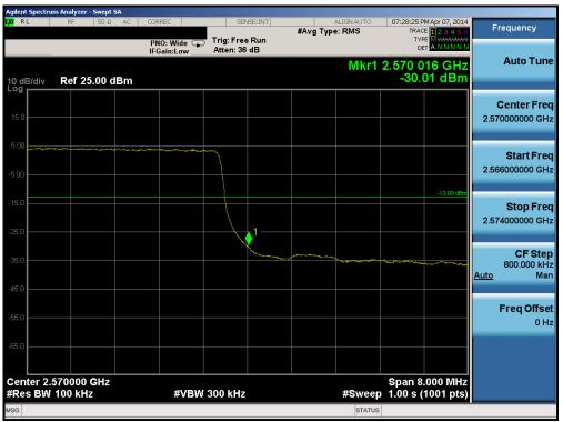
Plot 6-112. Upper Band Edge Plot (Band 7 – 10.0MHz QPSK – RB Size 50)
