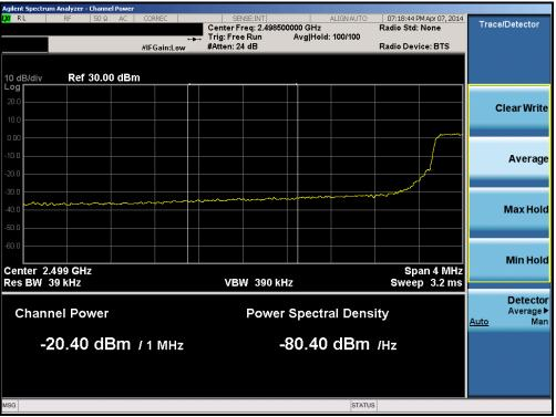
Plot 6-104. Lower Extended Band Edge Plot (Band 7 – 5.0MHz QPSK – RB Size 25)
