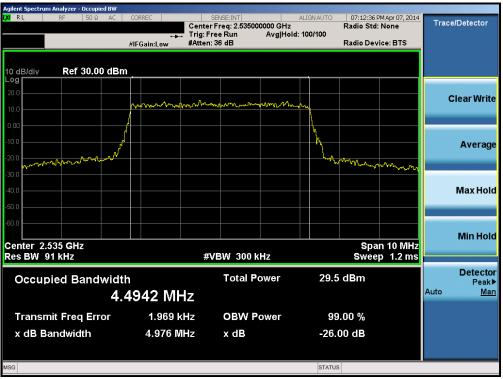
Plot 6-26. Occupied Bandwidth Plot (Band 7 – 5.0MHz 16-QAM – RB Size 25)
