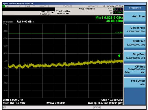
Plot 6-38. Conducted Spurious Plot (Band 17 – 10.0MHz QPSK – RB Size 1, RB Offset 0 – High Channel)
