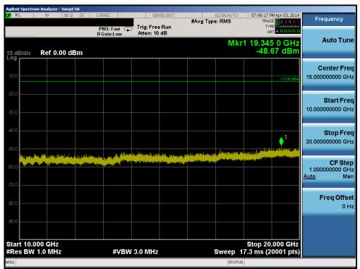
Plot 6-56. Conducted Spurious Plot (Band 2 – 5.0MHz QPSK – RB Size 1, RB Offset 0 – High Channel)
