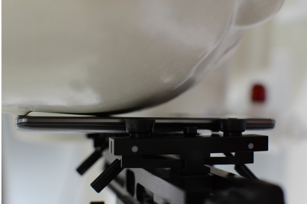
SAR Test Setup Photo 1 - Right Cheek
