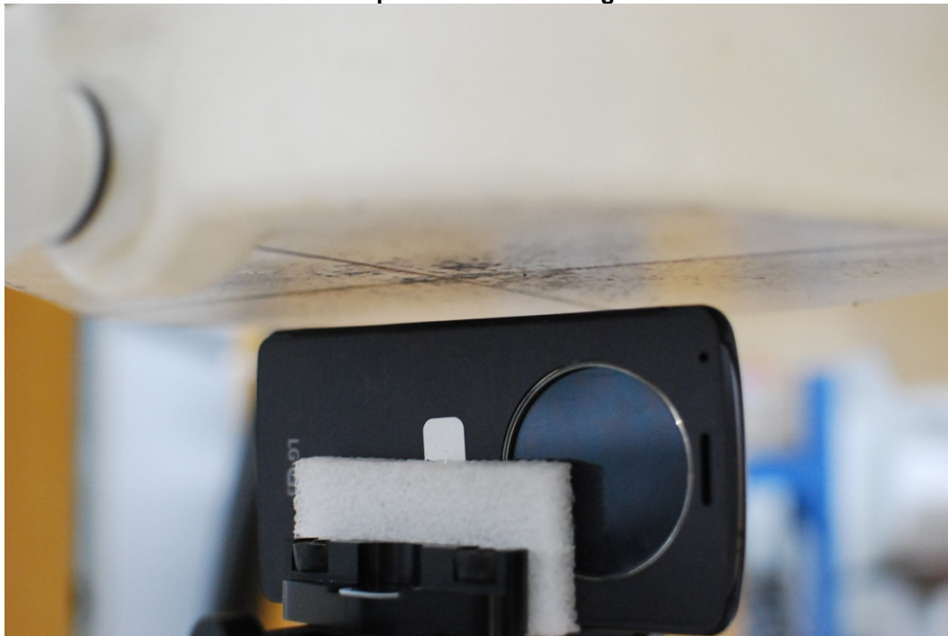
SAR Test Setup Photo 20 - Left Edge at 10 mm with WCC closed
