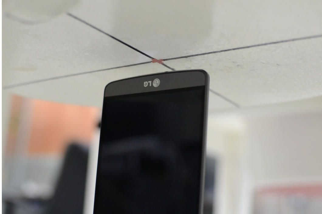
SAR Test Setup Photo 15 - Bottom at 10 mm
