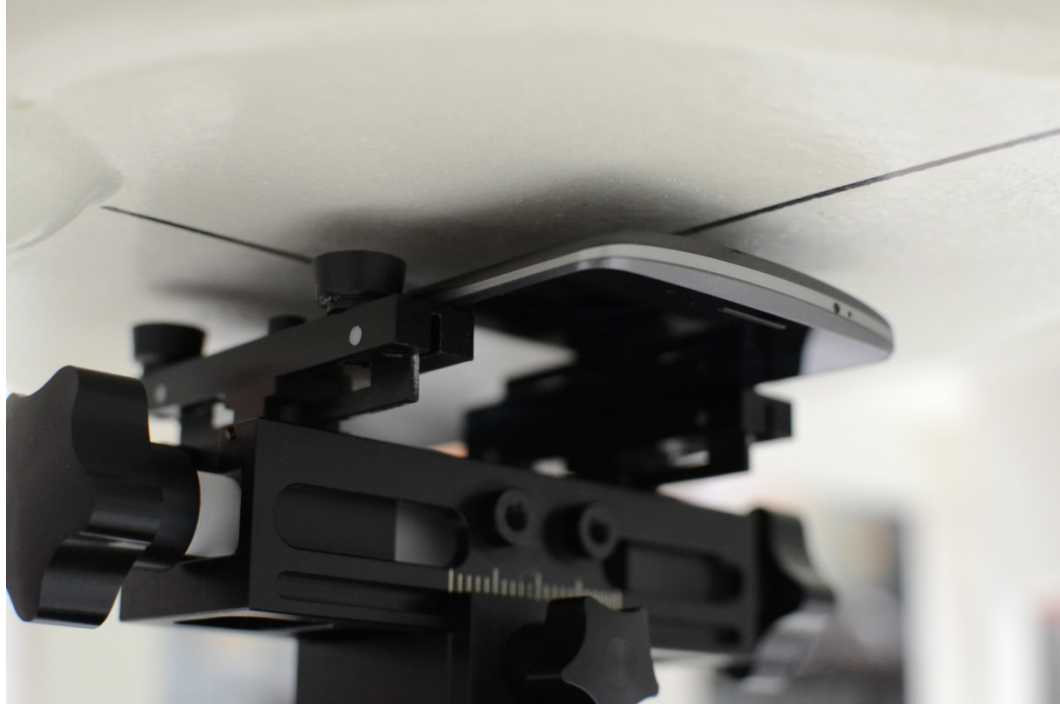
SAR Test Setup Photo 11 - Back at 10 mm
