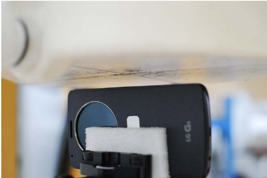
SAR Test Setup Photo 18 - Right Edge at 10 mm with WCC closed
