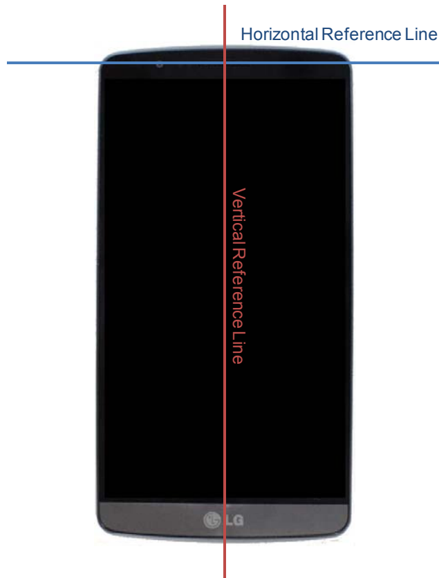
SAR Test Setup Photo 21 - Vertical and Horizontal Reference Lines
