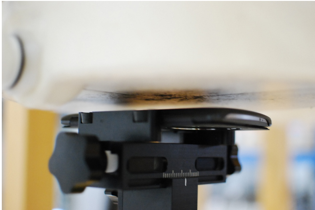
SAR Test Setup Photo 12 - Back at 10 mm with WCC closed
