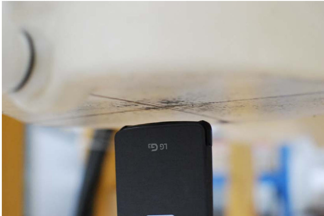
SAR Test Setup Photo 16 - Bottom at 10 mm with WCC closed
