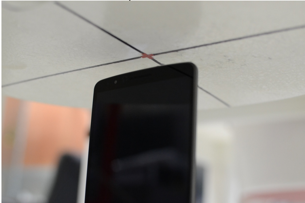
SAR Test Setup Photo 14 - Top at 10 mm
