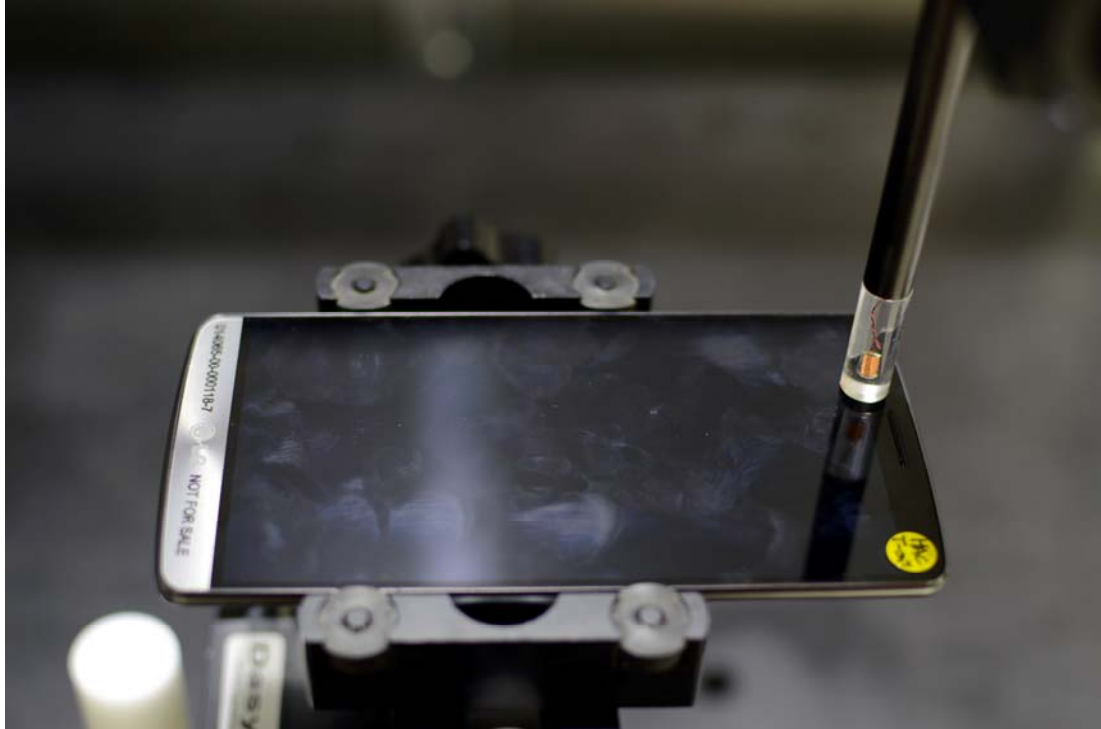
Figure 13-1 Test Setup for Wireless Device (Standard Battery Cover)
