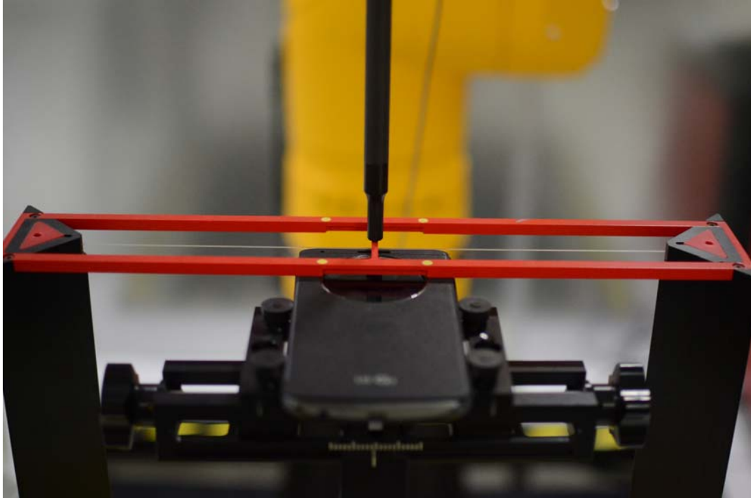
Figure 18-3 Ear Reference Point HAC Phantom Alignment, Wireless Charging Cover (Cover Closed)
