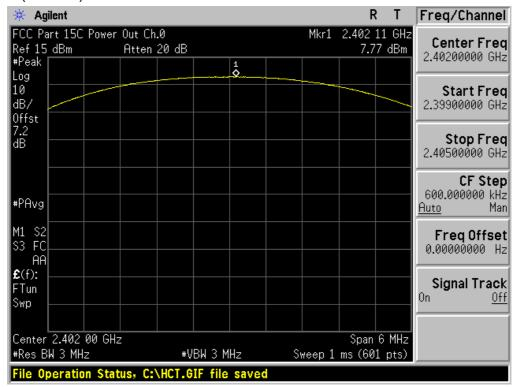
Test Plots (π/4DQPSK) Peak Power (Mid-CH)
