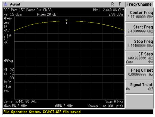
Test Plots (8DPSK) Peak Power (High-CH)
