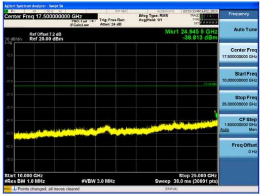
Test Plots ( $\pi$ /4DQPSK) - 10 GHz - 25 GHz (RBW:1 MHz, VBW: 3 MHz) Spurious Emission (Mid-CH)
