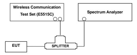
(Configuration of conducted Emission measurement)
