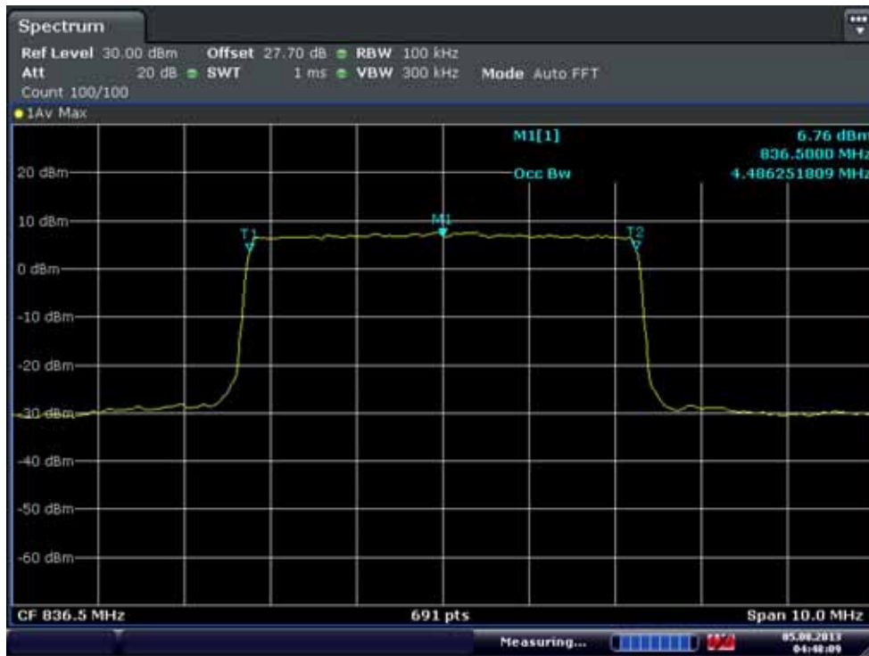
Occupied Bandwidth Plot (20525 ch_5 MHz_QPSK_RB Size 25)
