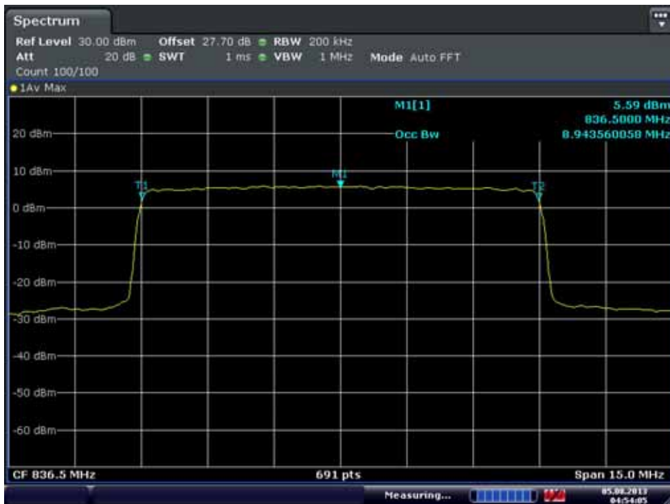
Occupied Bandwidth Plot (20525 ch_10 MHz_16-Q`AM_RB 50)
