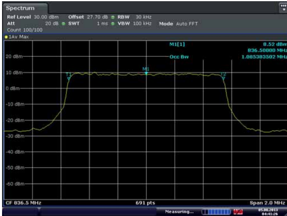
Occupied Bandwidth Plot (20525 ch_1.4 MHz_QPSK_RB Size 6)
