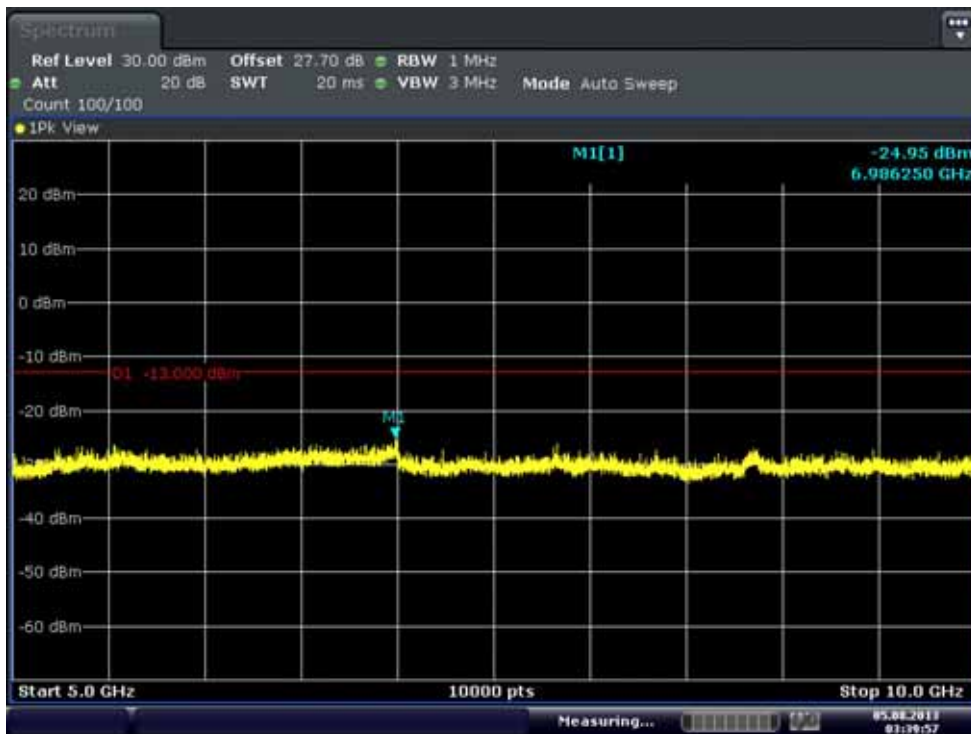
Conducted Spurious Plot_2 (20425 ch_5 MHz_QPSK_RB 25_0) -2
