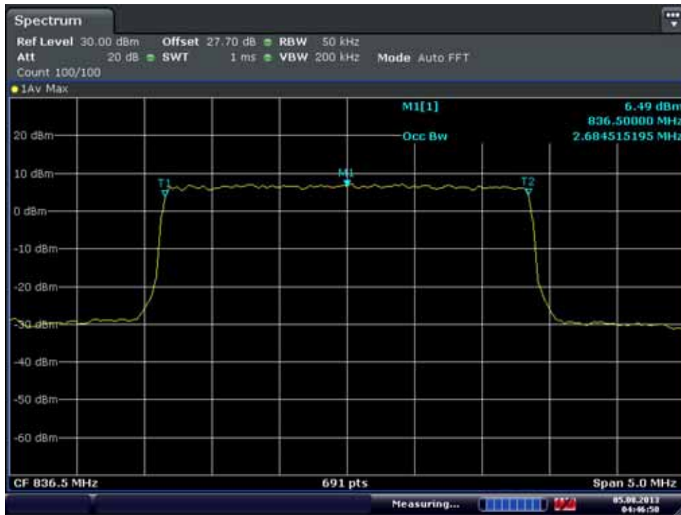
Occupied Bandwidth Plot (20525 ch_3 MHz_QPSK_RB 15)
