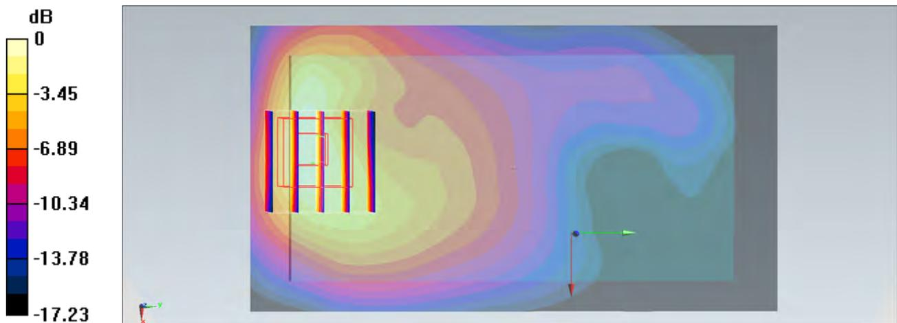
0 dB =  $0.479 \text{ W/kg} = -3.20 \text{ dBW/kg}$
