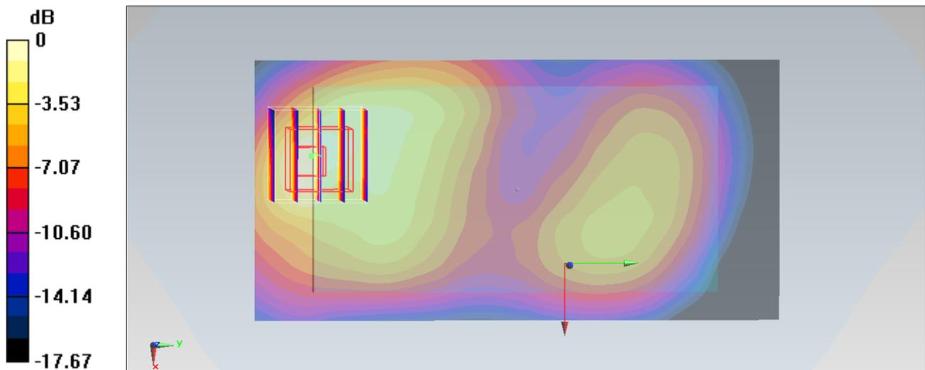
0 dB =  $0.595 \text{ mW/g}$  =  $-4.51 \text{ dB mW/g}$
