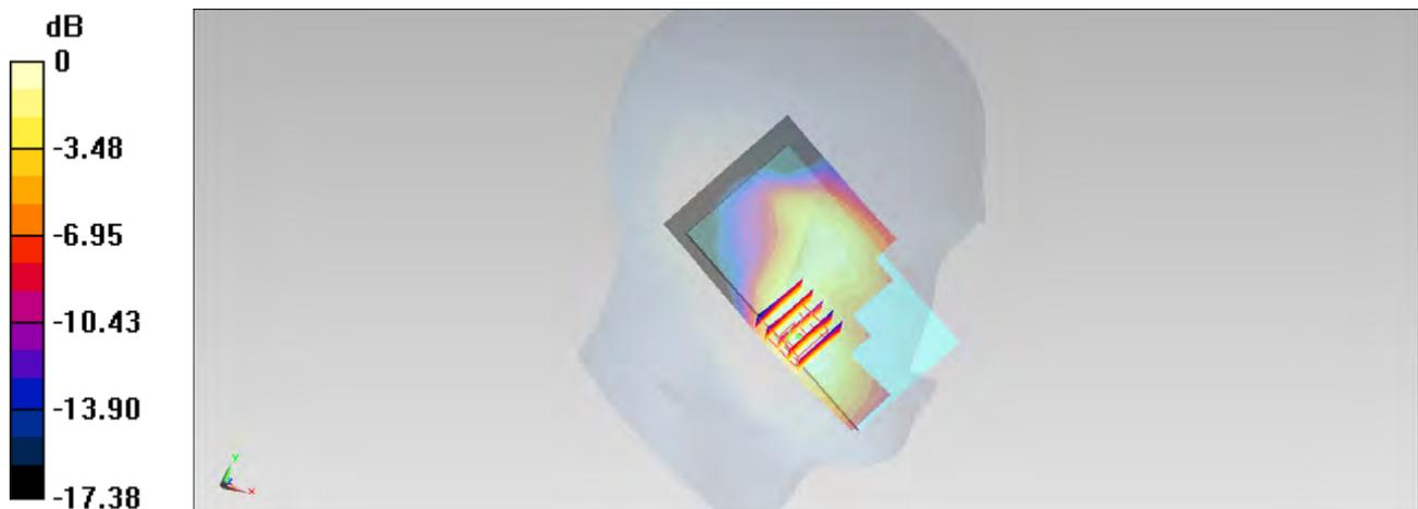
0 dB =  $0.0892 \text{ W/kg}$  =  $-10.50 \text{ dBW/kg}$
