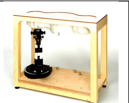
Fig 5.9 Photo of SAM Phantom
