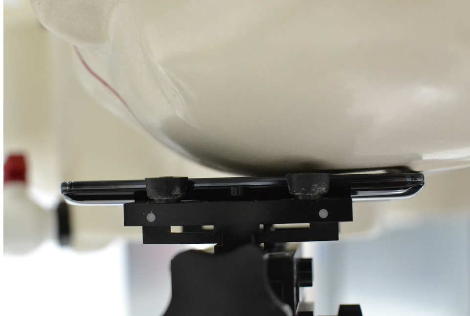
SAR Test Setup Photo 3: Left Cheek
