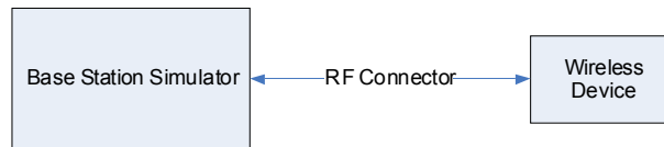
Figure 9-2 Power Measurement Setup
