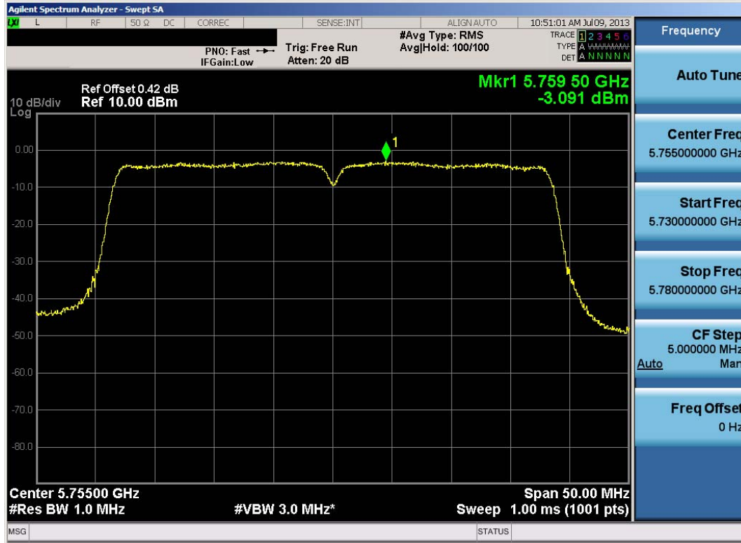
Plot 6-73. Peak Power Spectral Density Plot (40MHz BW 802.11n (UNII Band 4) – Ch. 151)
