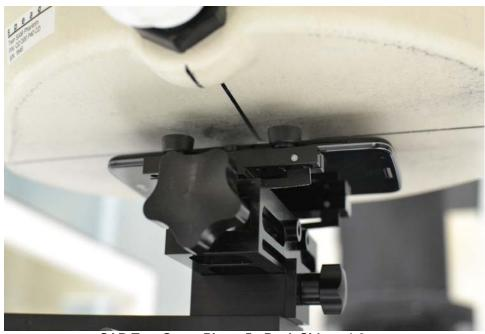
SAR Test Setup Photo 5 - Back Side at 1.0 cm
