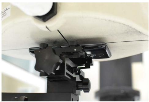
SAR Test Setup Photo 6 - Front Side at 1.0 cm
