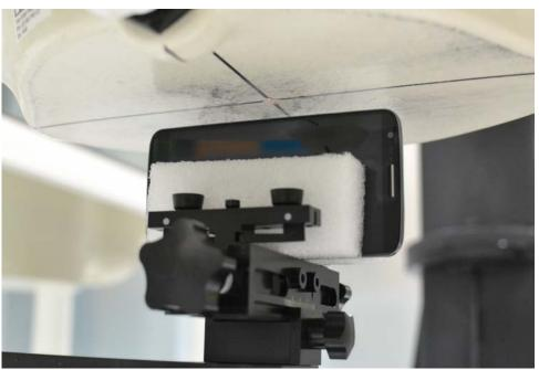
SAR Test Setup Photo 10 - Left Edge at 1.0 cm
