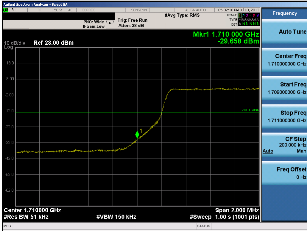
Plot 9-1. Lower Band Edge Plot (5.0MHz QPSK – RB Size 25)
