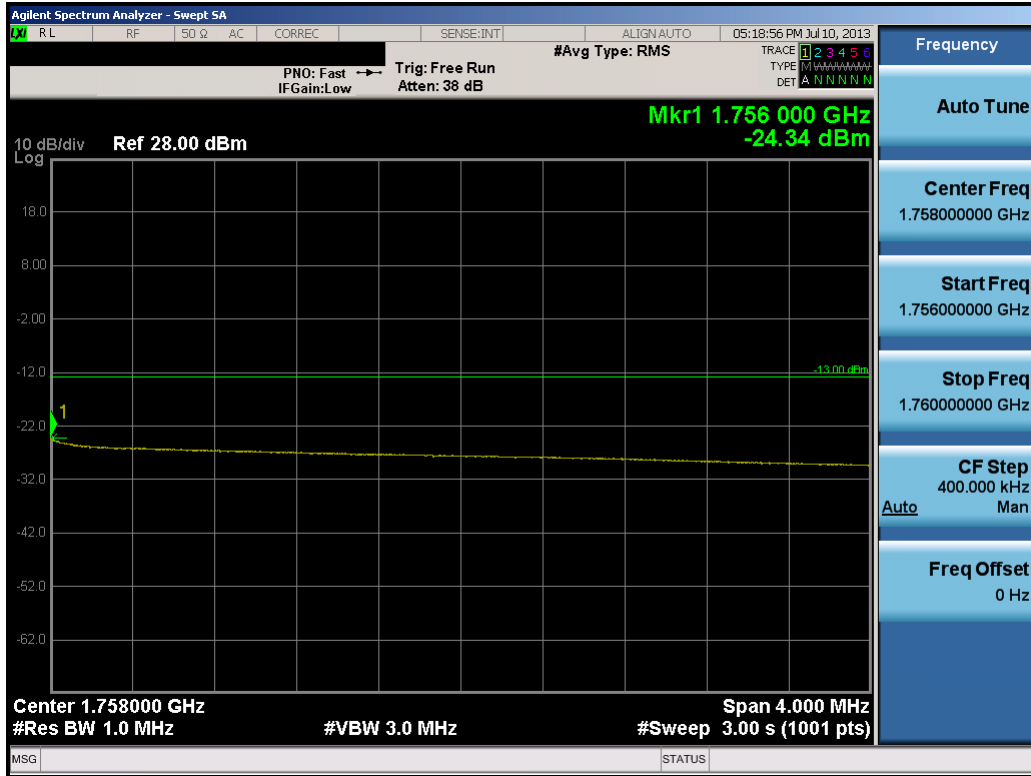
Plot 9-26. Upper Extended Band Edge Plot (10.0MHz QPSK – RB Size 50)
