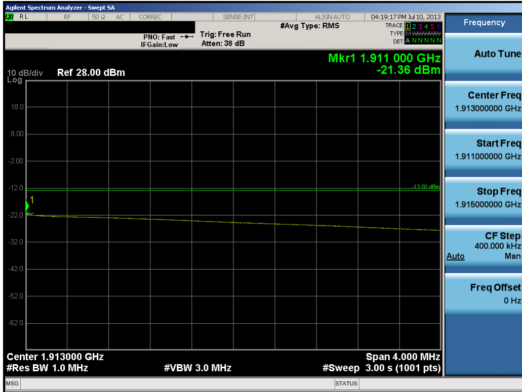
Plot 10-26. Upper Extended Band Edge Plot (10.0MHz QPSK – RB Size 50)
