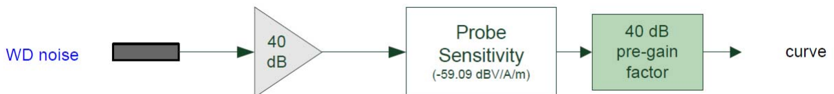
Figure 6-2 Audio Band Magnetic Curve Measurement Block Diagram
