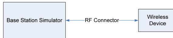
Figure 9-1 Power Measurement Setup
