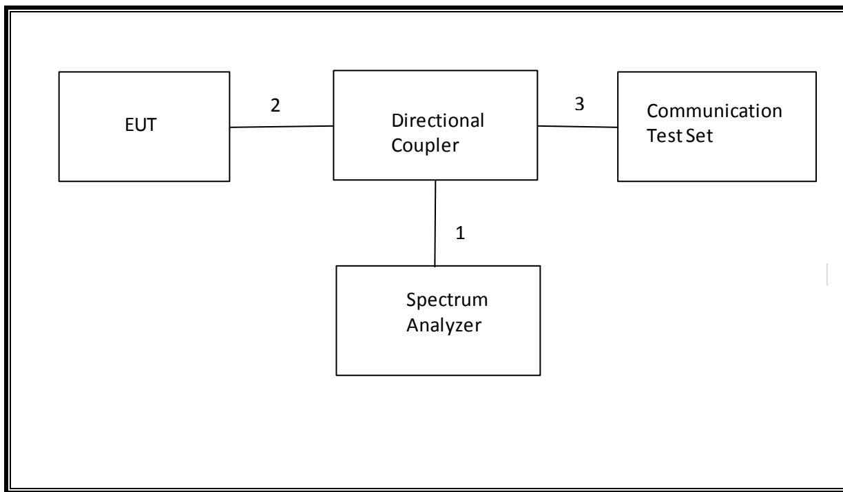
**SETUP DIAGRAM FOR TESTS (RADIATED TEST SETUP)**
