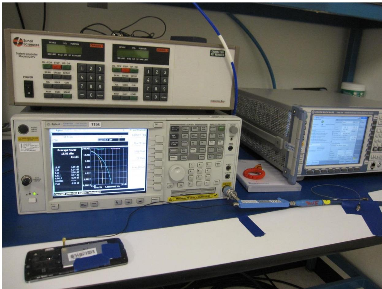
**RADIATED RF MEASUREMENT SETUP FOR PORTABLE CONFIGURATION**
