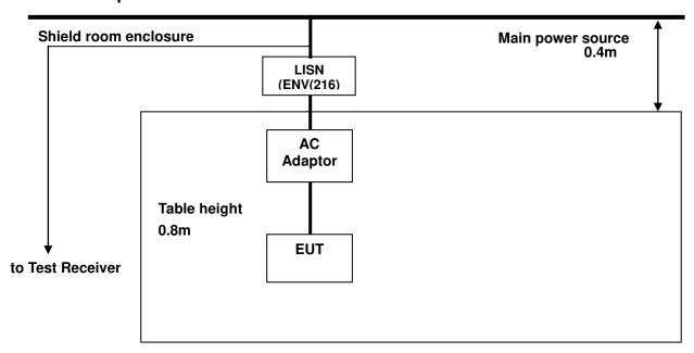
6.1.1. Actual equipment used for AC Power Line Conducted Emission
