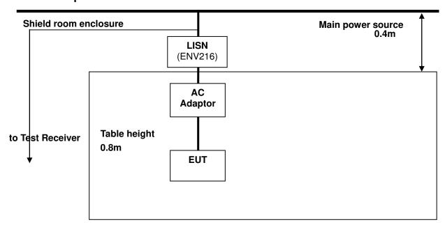
6.1.1. Actual equipment used for AC Power Line Conducted Emission
