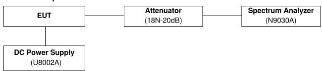
5.1.1. Actual equipment used for Power Spectral Density measurement
