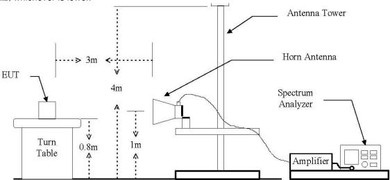
2.1.1.1. Actual equipment used for Radiated spurious Emissions
