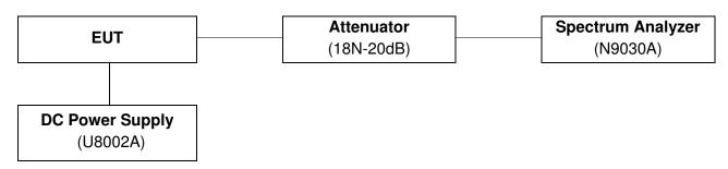
2.1.2.1. Actual equipment used for Conducted Spurious Emissions
