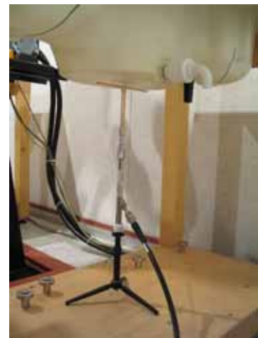
Photo of the dipole Antenna
