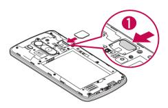
3 Insert the battery into place by aligning the gold contacts on the phone and the battery (1) and pressing it down until it clicks into place (2).
