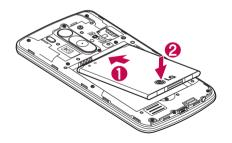
4 Align the battery cover over the battery compartment (1) and press it down until it clicks into place (2).
