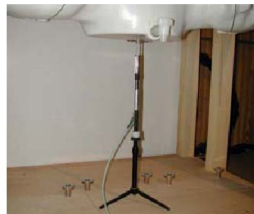
Figure 11.1 Dipole Verification Test Setup Diagram & Photo
