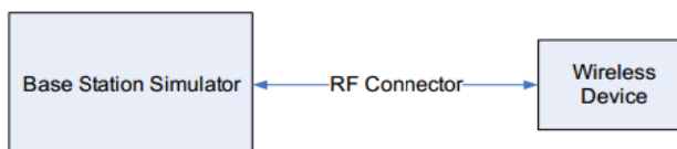
Figure 10.1 Power Measurement Setup
