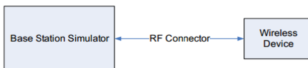
Figure 10.1 Power Measurement Setup
