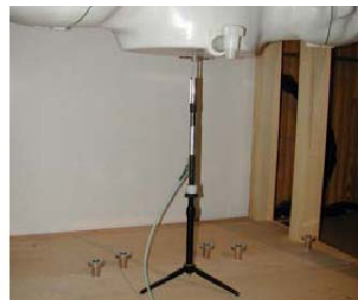
Figure 11.1 Dipole Verification Test Setup Diagram & Photo
