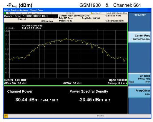
PAPR (dB) =  $P_{Pk}$  (dBm) -  $P_{Avq}$  (dBm) = 30.70dBm - 30.44 dBm = 0.26 dB
