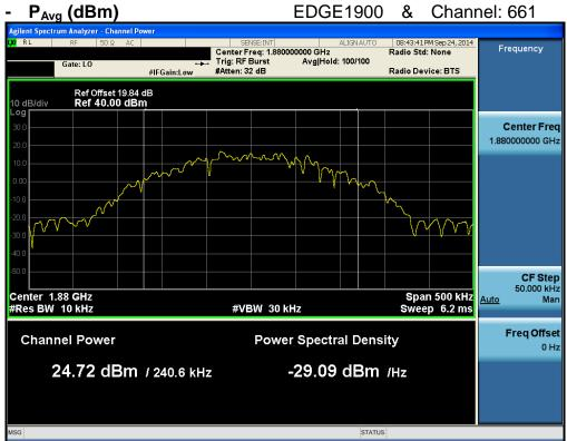
$PAR (dB) = P_{Pk} (dBm) - P_{Avq} (dBm) = 30.67 dBm - 24.72 dBm = 5.95 dB$
