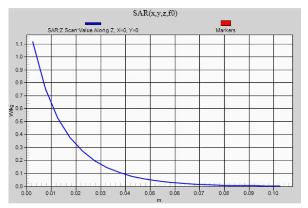
Frequency: 836.6 MHz; Duty Cycle: 1:8.00018; Room Ambient Temperature: 24.0°C; Liquid Temperature: 23.0°C Medium parameters used (interpolated): f = 836.6 MHz;  $\sigma = 0.941$  S/m;  $\epsilon_r = 42.471$ ;  $\rho = 1000$  kg/m<sup>3</sup> DASY5 Configuration:
