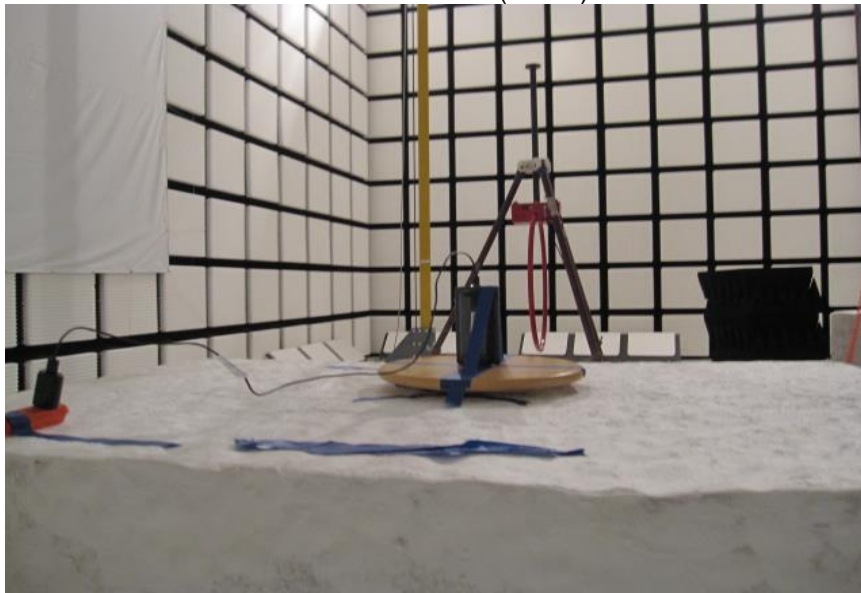
RADIATED EMISSIONS BELOW 30MHz (BACK)
