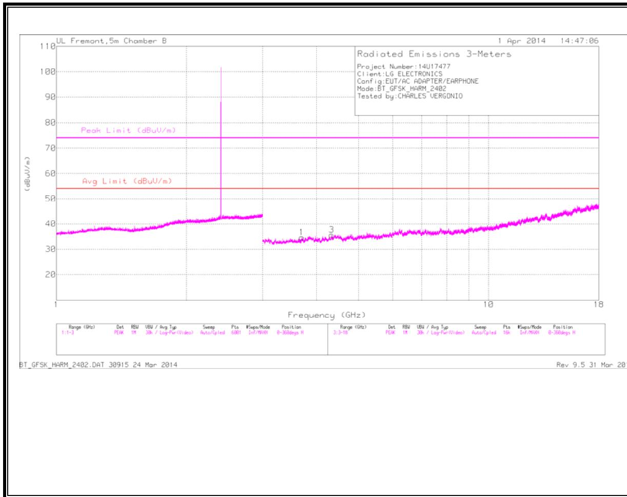
Note: Emission was scanned up to 26GHz; No emissions were detected above the noise floor which was at least 20dB below the specification limit.
