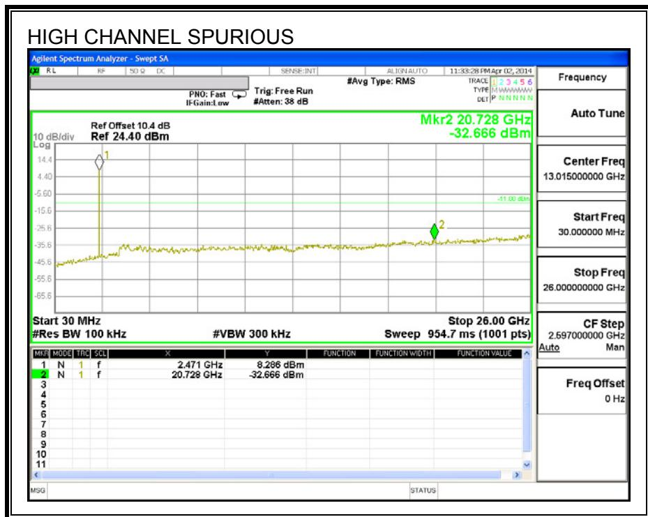
**SPURIOUS BANDEDGE EMISSIONS WITH GFSK HOPPING ON**
