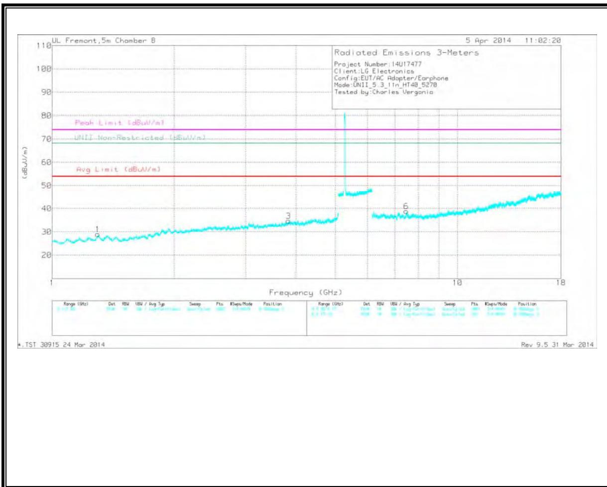
Note: Emission was scanned up to 40GHz; No emissions were detected above the noise floor which was at least 20dB below the specification limit.
