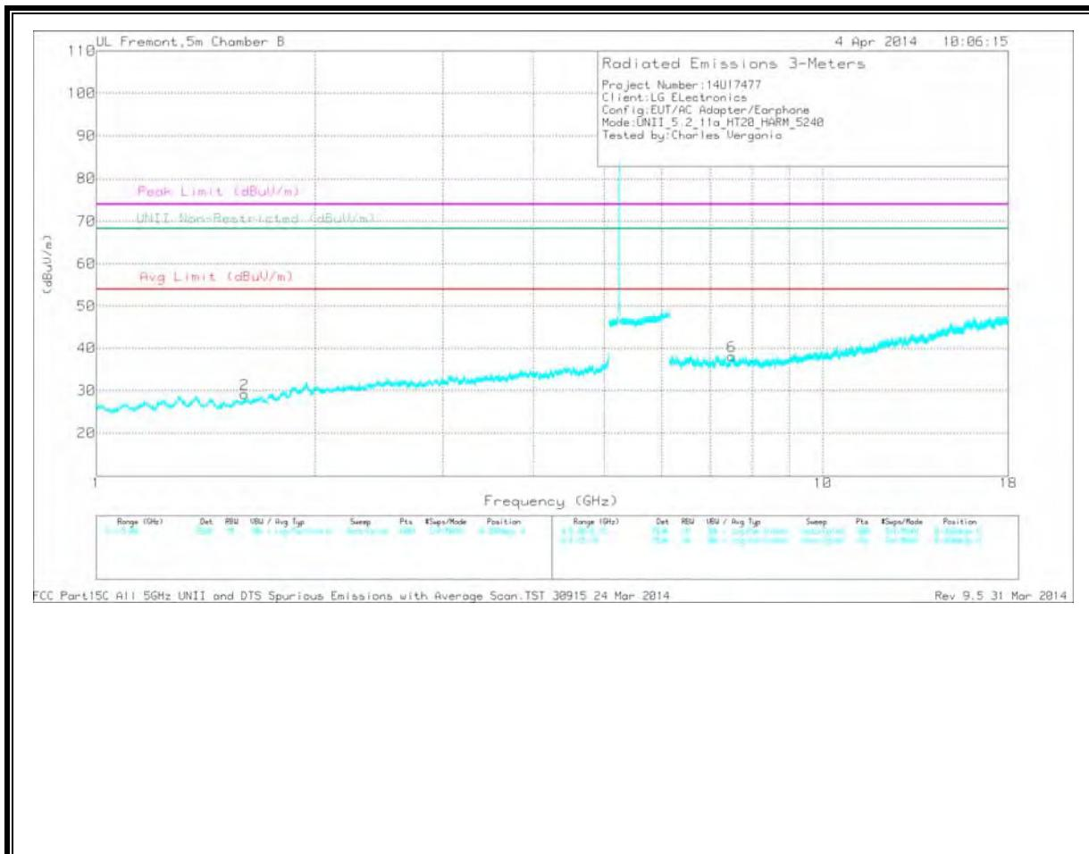
Note: Emission was scanned up to 40GHz; No emissions were detected above the noise floor which was at least 20dB below the specification limit.
