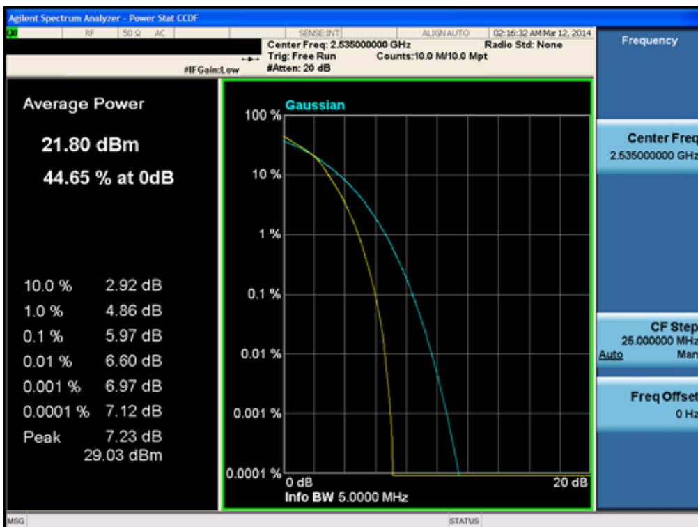
Peak to Average Ratio Plot (5MHz Ch.21100 16-QAM RB 25)
