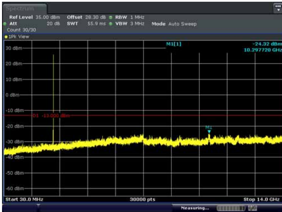
Conducted Spurious Plot 1 (5MHz Ch.20775 QPSK RF 1, Offset 0)
