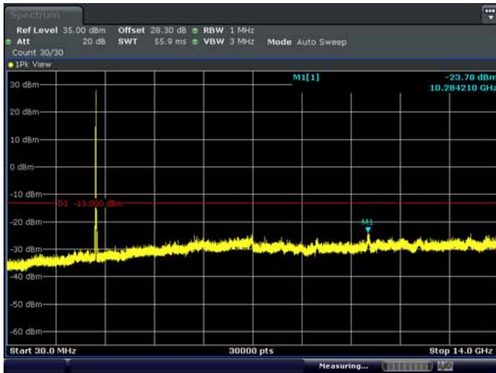
Conducted Spurious Plot 1 (20MHz Ch.21350 QPSK RF 1, Offset 0)
