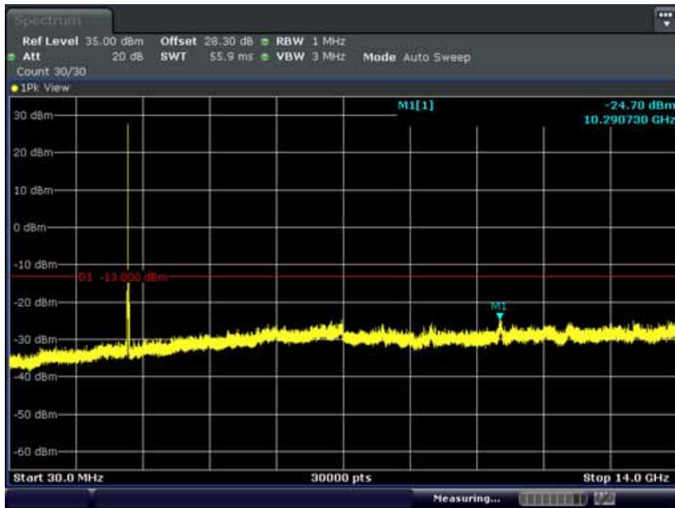
Conducted Spurious Plot 1 (20MHz Ch.20850 QPSK RF 1, Offset 0)
