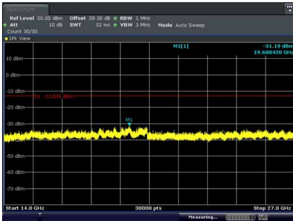
Conducted Spurious Plot 2 (10MHz Ch.21100 QPSK RF 1, Offset 0)
