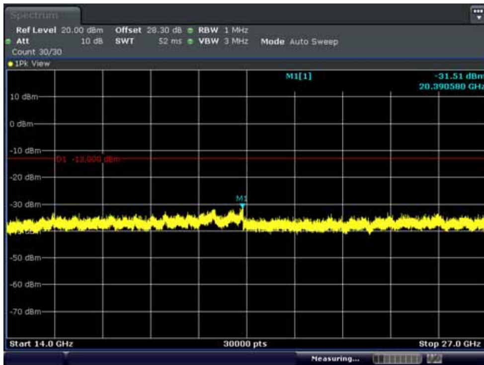
Conducted Spurious Plot 2 (5MHz Ch.21425 QPSK RF 1, Offset 0)
