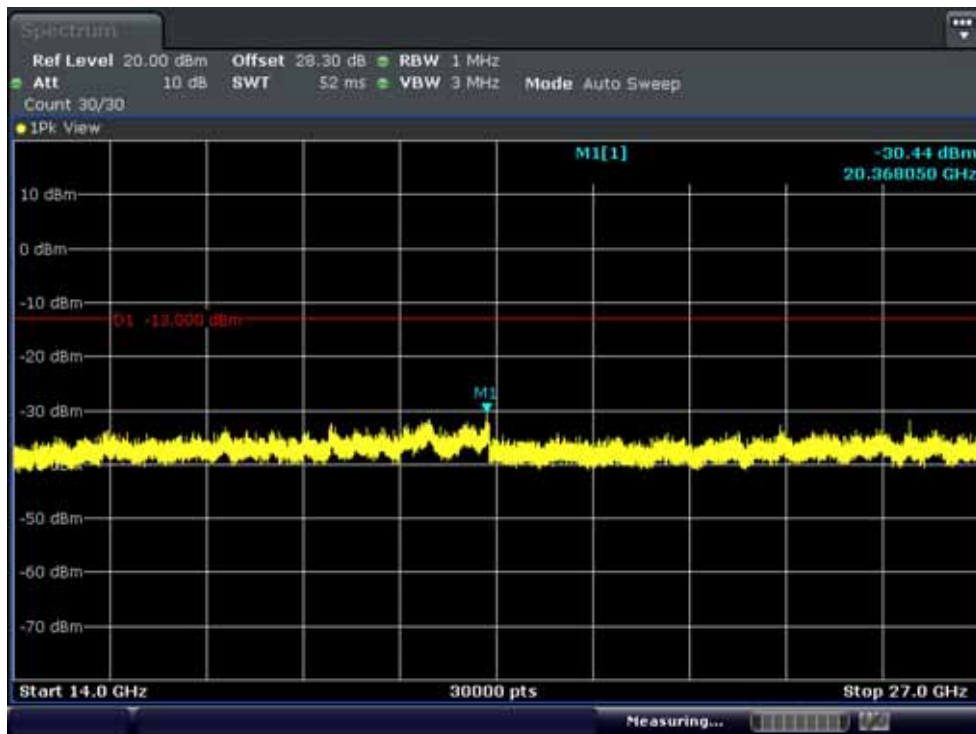
Conducted Spurious Plot 2 (20MHz Ch.20850 QPSK RF 1, Offset 0)
