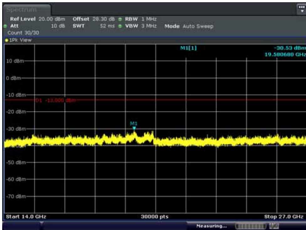
Conducted Spurious Plot 2 (5MHz Ch.20775 QPSK RF 1, Offset 0)
