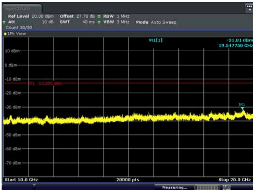
Band 4: Conducted Spurious Plot 2 (5MHz QPSK - RB Size 1, RB Offset 0 - High Band 4: Channel)
