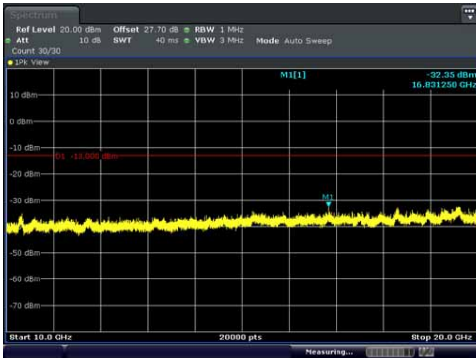
Band 4: Conducted Spurious Plot 2 (5MHz QPSK - RB Size 1, RB Offset 0 - Mid Band 4: Channel)
