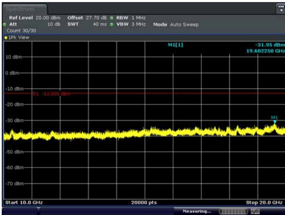
Band 4: Conducted Spurious Plot 2 (10MHz QPSK - RB Size 1, RB Offset 0 - Mid Band 4: Channel)
