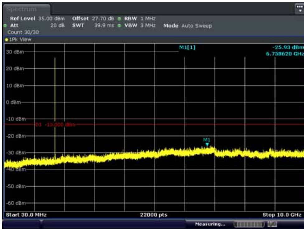
Band 4: Conducted Spurious Plot 1 (1.4MHz QPSK - RB Size 1, RB Offset 0 - Low Band 4: Channel)
