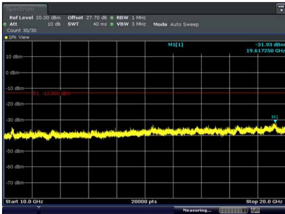
Band 4: Conducted Spurious Plot 2 (20MHz QPSK - RB Size 1, RB Offset 0 - High Band 4: Channel)
