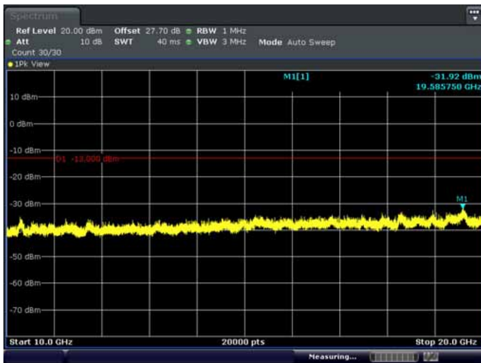
Band 4: Conducted Spurious Plot 2 (10MHz QPSK - RB Size 1, RB Offset 0 - Low Band 4: Channel)
