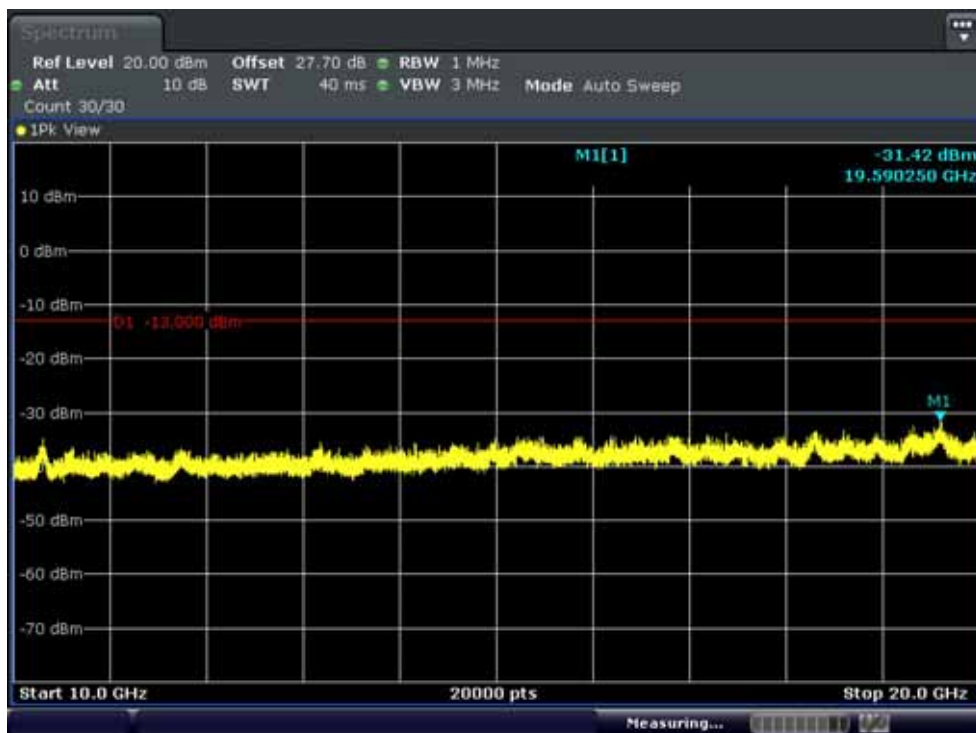
Band 4: Conducted Spurious Plot 2 (3MHz QPSK - RB Size 1, RB Offset 0 - Low Band 4: Channel)
