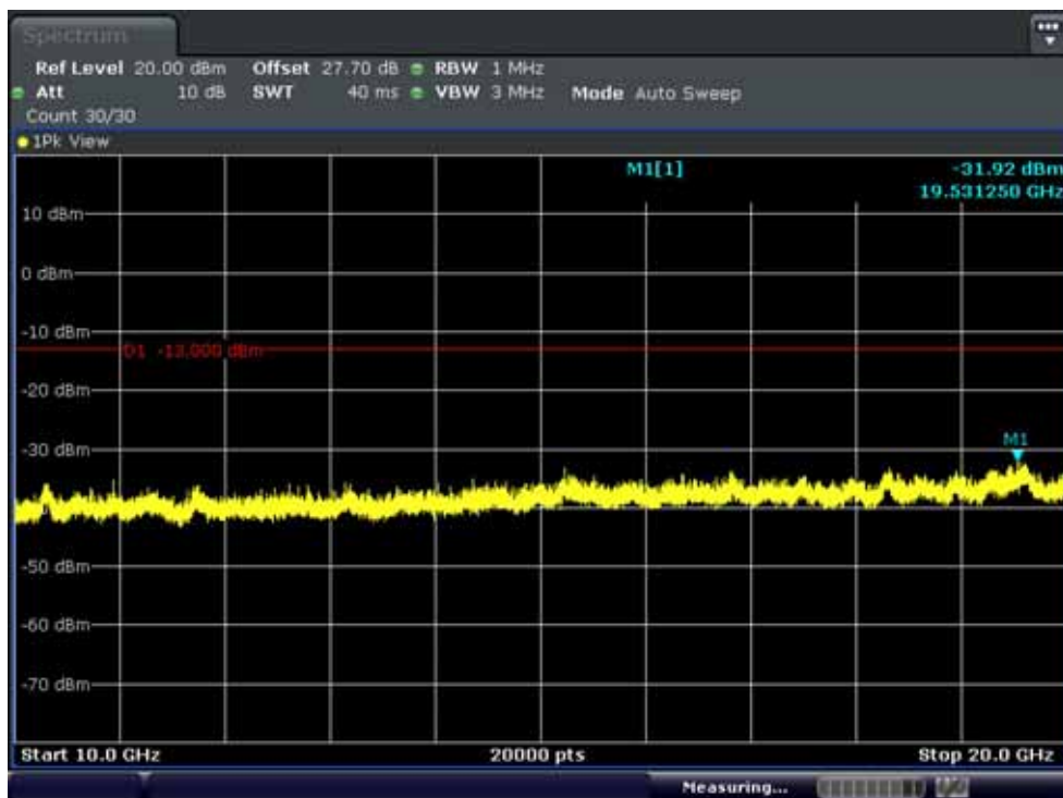
Band 4: Conducted Spurious Plot 2 (20MHz QPSK - RB Size 1, RB Offset 0 - Mid Band 4: Channel)
