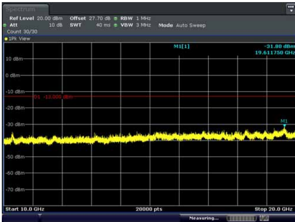
Band 4: Conducted Spurious Plot 2 (3MHz QPSK - RB Size 1, RB Offset 0 - High Band 4: Channel)
