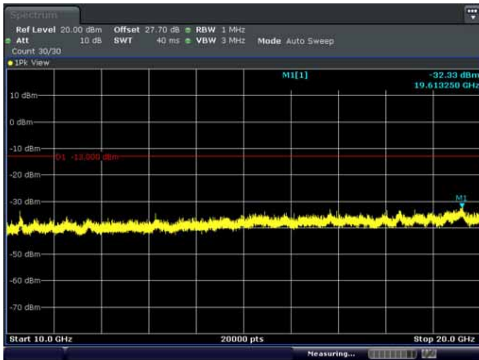
Band 4: Conducted Spurious Plot 2 (1.4MHz QPSK - RB Size 1, RB Offset 0 - Low Band 4: Channel)
