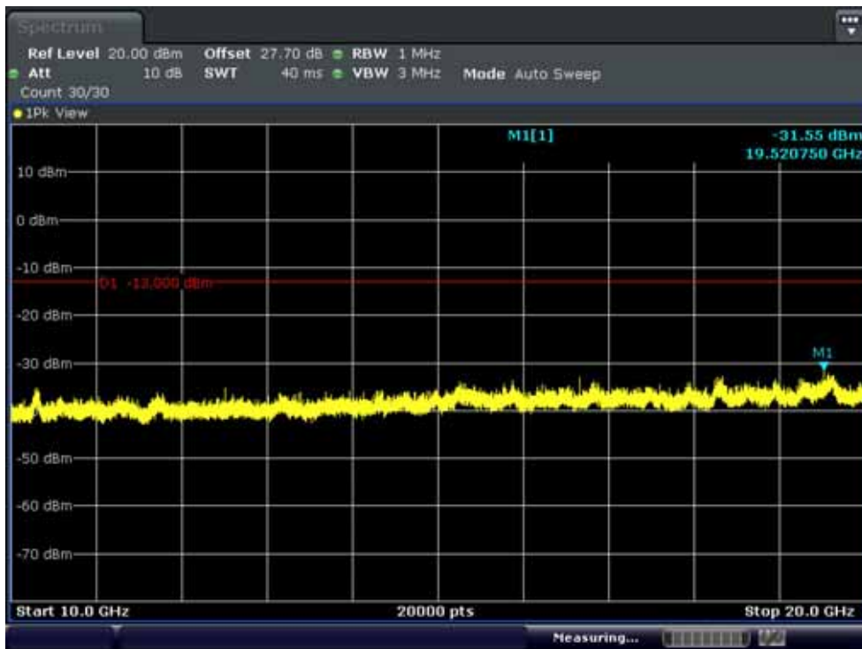
Band 4: Conducted Spurious Plot 2 (20MHz QPSK - RB Size 1, RB Offset 0 - Low Band 4: Channel)
