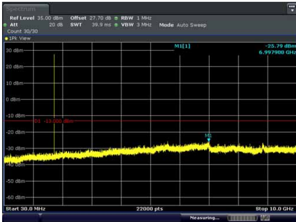
Band 4: Conducted Spurious Plot 1 (1.4MHz QPSK - RB Size 1, RB Offset 0 - Mid Band 4: Channel)
