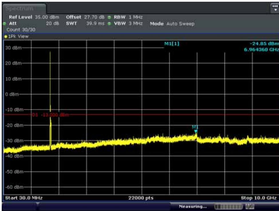
Band 4: Conducted Spurious Plot 1 (20MHz QPSK - RB Size 1, RB Offset 0 - Low Band 4: Channel)
