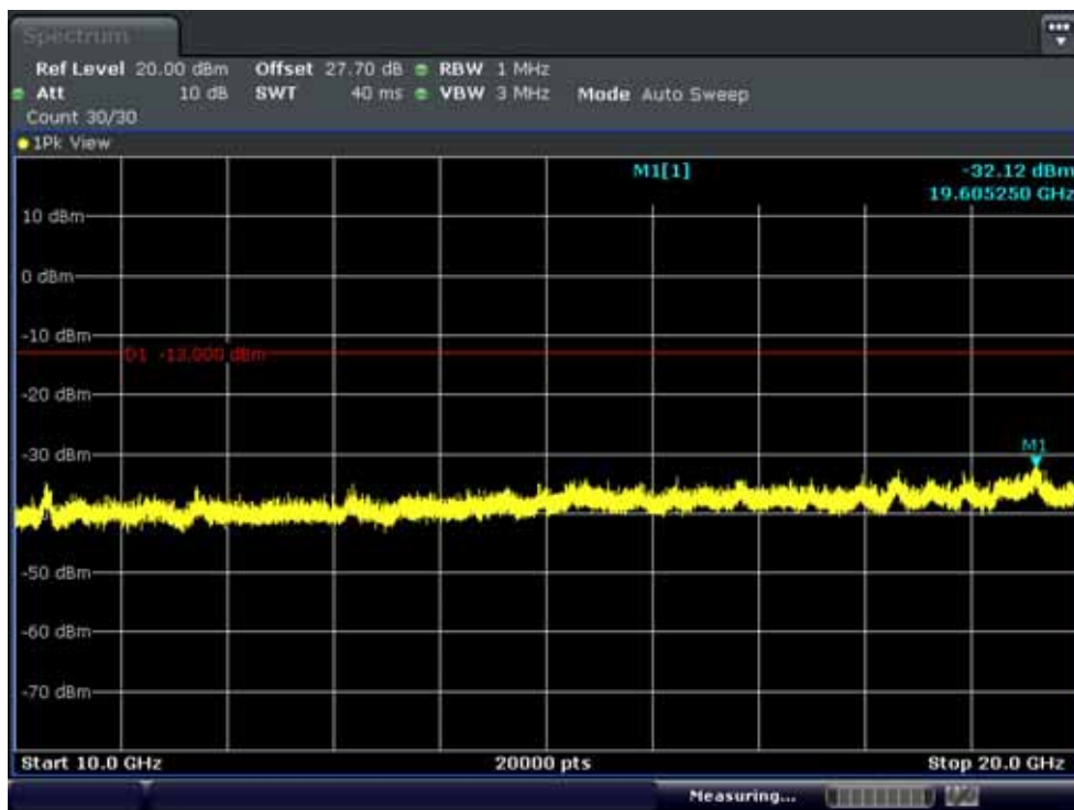
Band 4: Conducted Spurious Plot 2 (10MHz QPSK - RB Size 1, RB Offset 0 - High Band 4: Channel)
