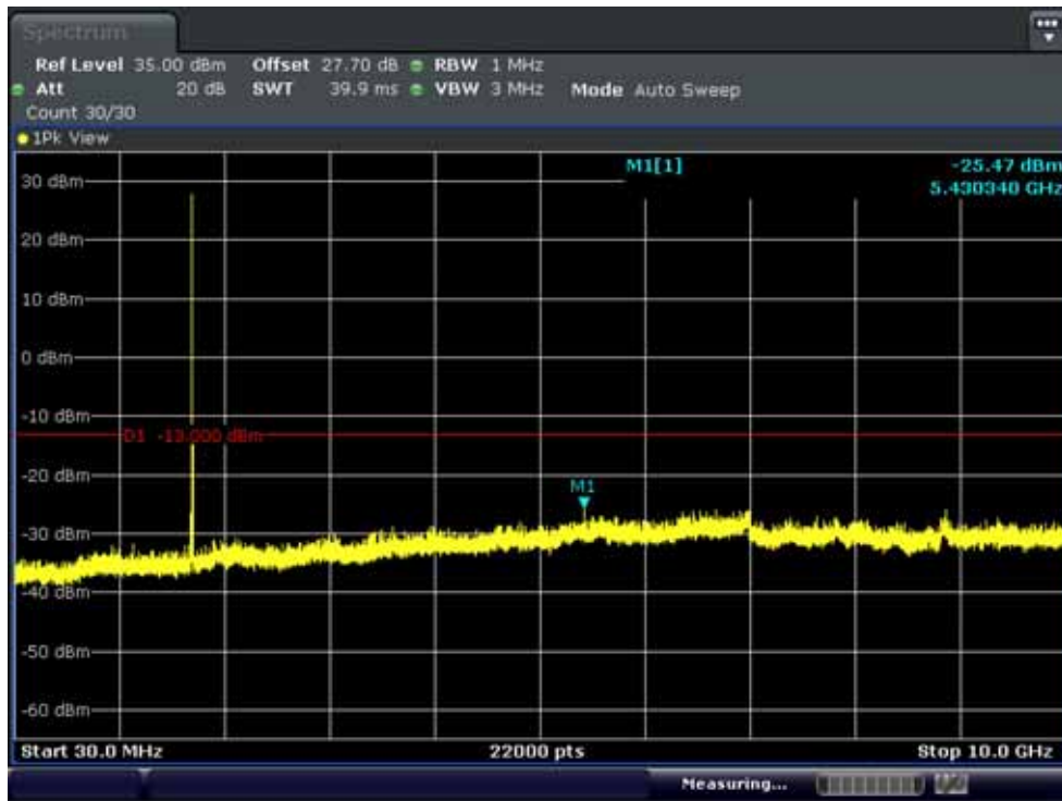
Band 4: Conducted Spurious Plot 1 (5MHz QPSK - RB Size 1, RB Offset 0 - Low Band 4: Channel)
