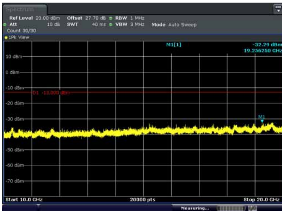
Band 4: Conducted Spurious Plot 2 (3MHz QPSK - RB Size 1, RB Offset 0 - Mid Band 4: Channel)
