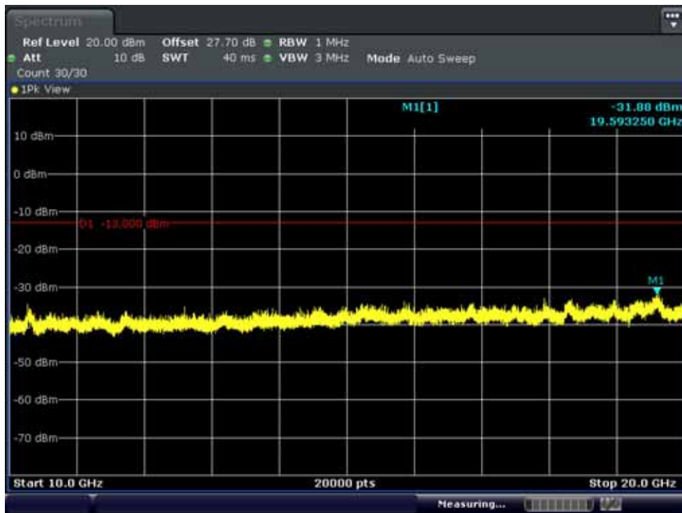
Band 4: Conducted Spurious Plot 2 (15MHz QPSK - RB Size 1, RB Offset 0 - Mid Band 4: Channel)
