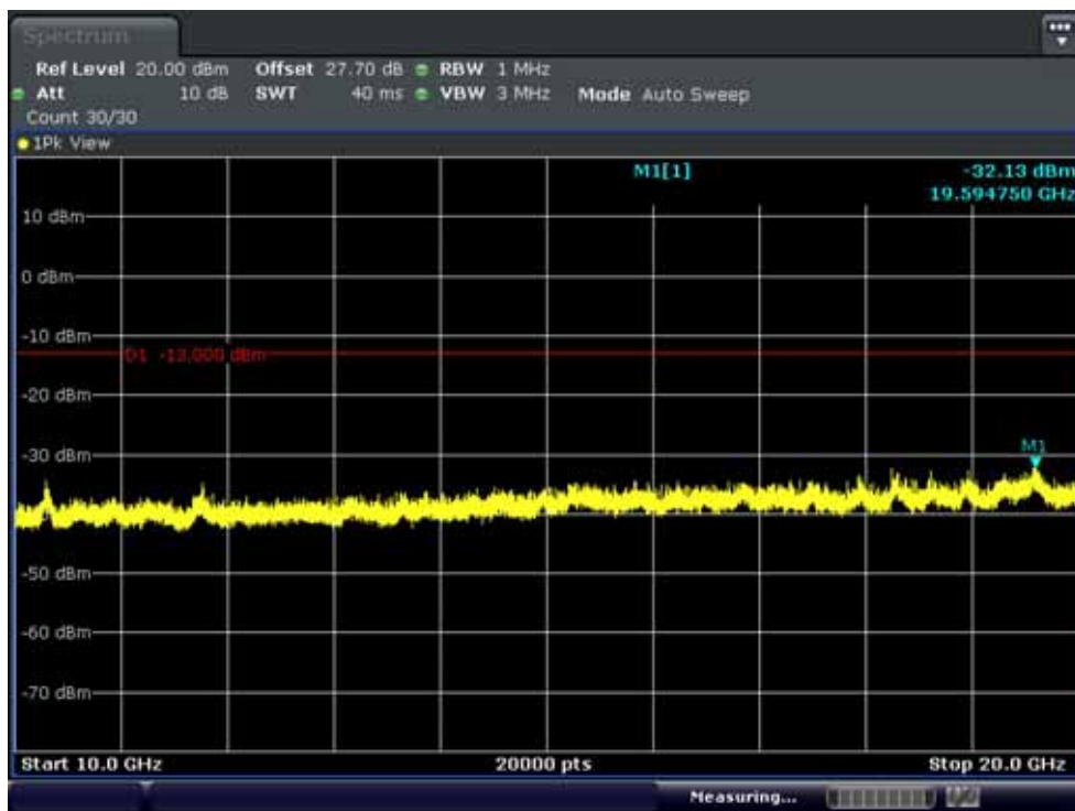
Band 4: Conducted Spurious Plot 2 (15MHz QPSK - RB Size 1, RB Offset 0 - High Band 4: Channel)
